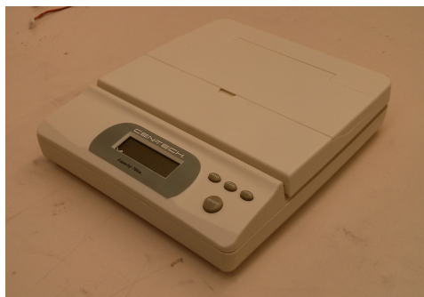
Figure 5.7: This figure shows the 70 lb digital scale from which the strain gauges were removed.
