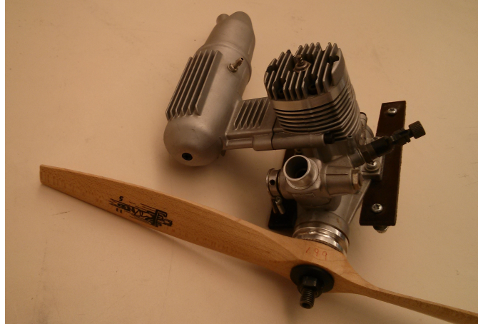
Figure 3.1: Front view of typical model 2-stroke engine.
