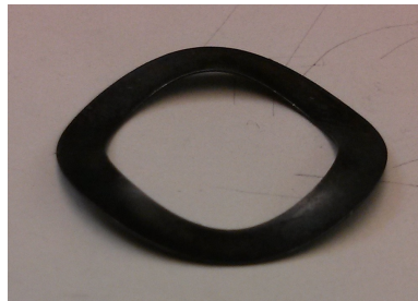
Figure 5.35: This figure shows the wave spring behind the front bearing.
