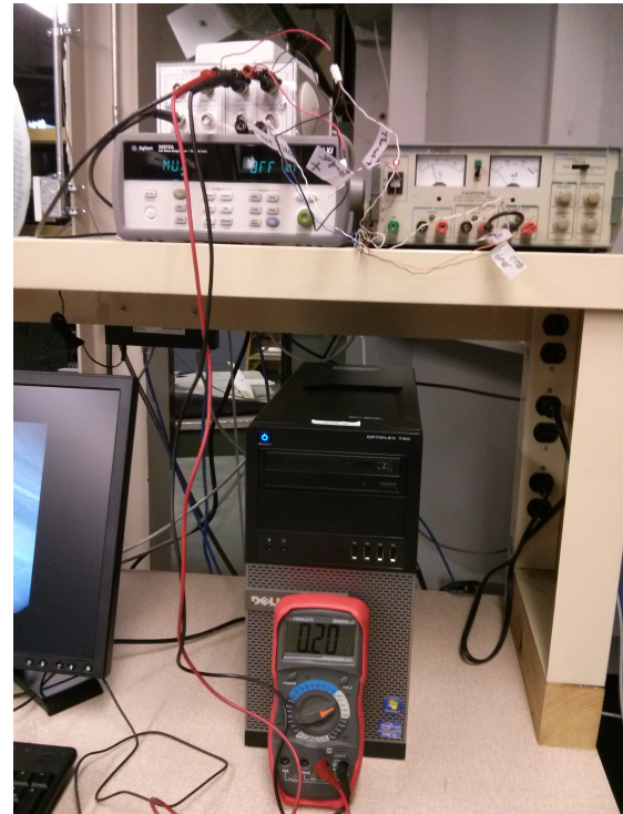
(b) A figure showing the zero reading on a voltmeter for the thrust strain gauges.
