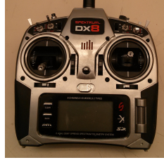
Figure 5.2: This figure shows the DX8 transmitter.
