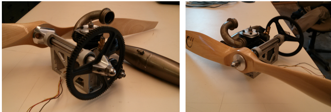
Figure 5.52: Front and rear view of the finalized geared power plant.
