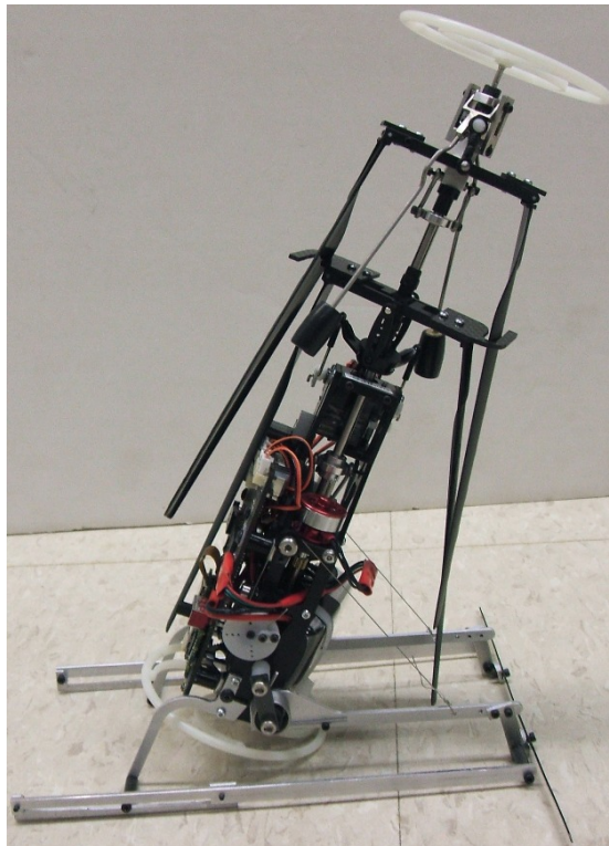
Figure B.8: A prototype of Hybrid V1.1 midway through transformation. The upper rotor is retained close to the robot's body as it tips down, keeping the lower rotor folded as well.
