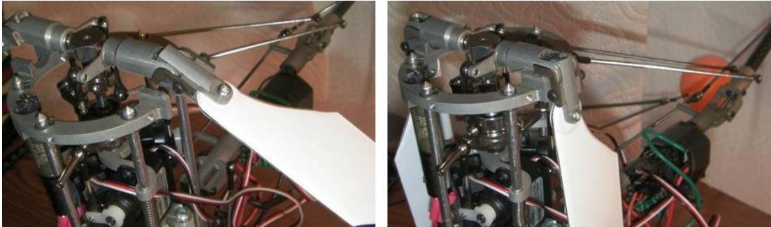
Figure 2.17: Photos of the prototype’s rotor folding mechanism in the fully extended (left) and fully retracted positions. This prototype is equipped with heavier rotor blades than the mechanism was designed for, so they “droop” somewhat even when fully extended. This aids the function of the folding mechanism by improving its pressure angle at the early stage of operation. Centrifugal force extends the rotors fully when the rotor head is spun up.
