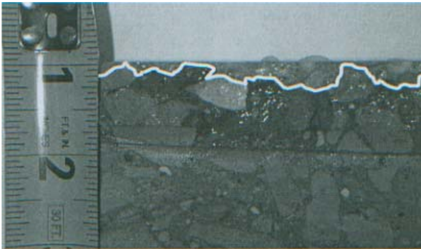
Figure 4: Depth of penetration measurement (Pincheira 2005)
