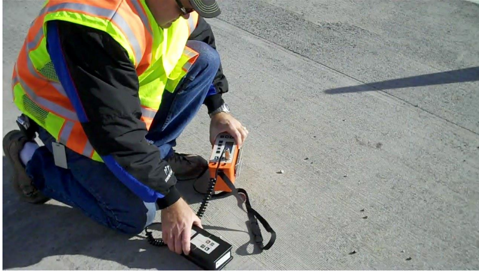
Figure 2-4. Example eddy current magnetic based device (pachometer).
