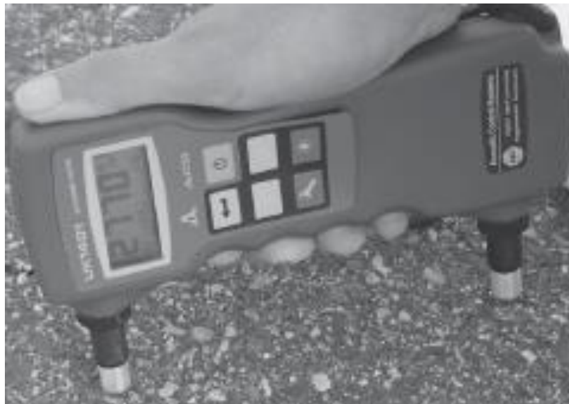
Figure 2-11. UK1401 ultrasonic pulse velocity device (Khazanovich et al., 2005).
