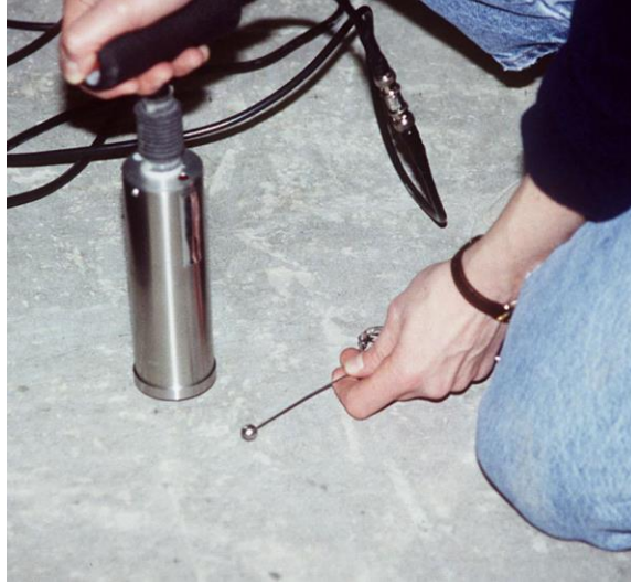
Figure 2-8. Impact echo setup with a steel ball mounted on a steel spring rod (Carino, 2001).
