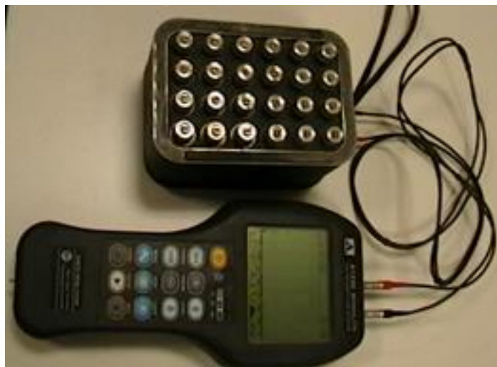
Figure 2-13. A1220 ultrasonic pulse-echo device.
