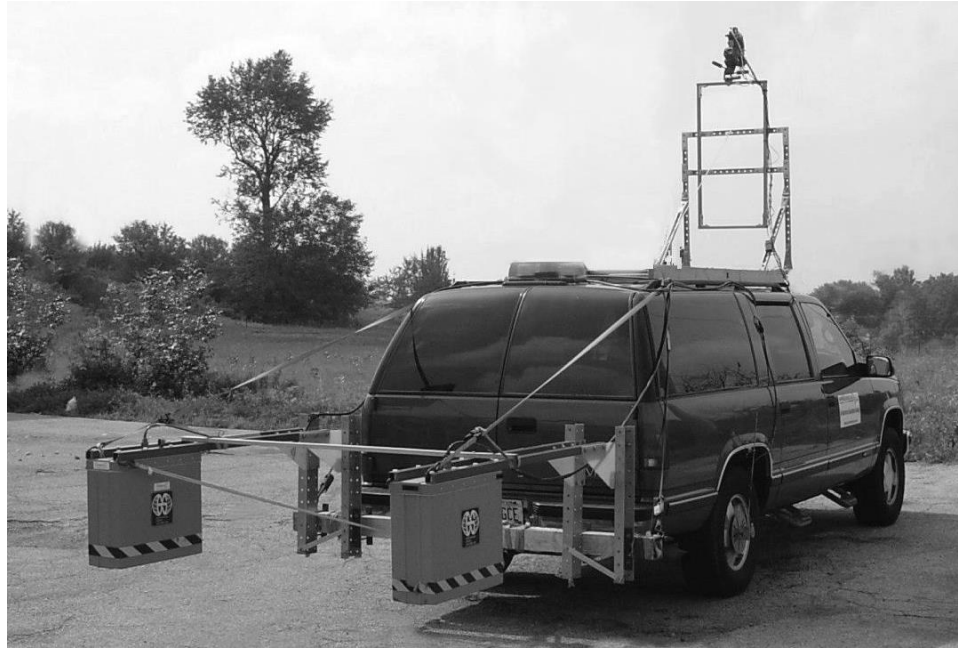
Figure 2-2. Air coupled GPR mounted on a van for highway speed measurements (Maser, 2000).
