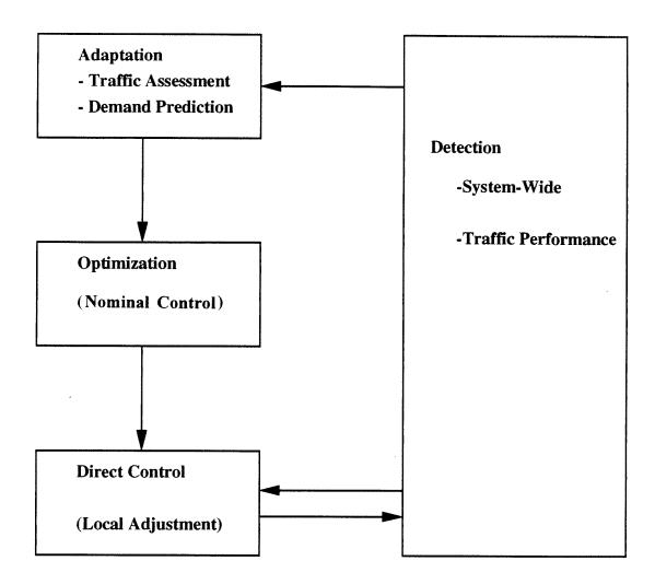
Figure 1.1. Hierarchical Control System for Freeways
