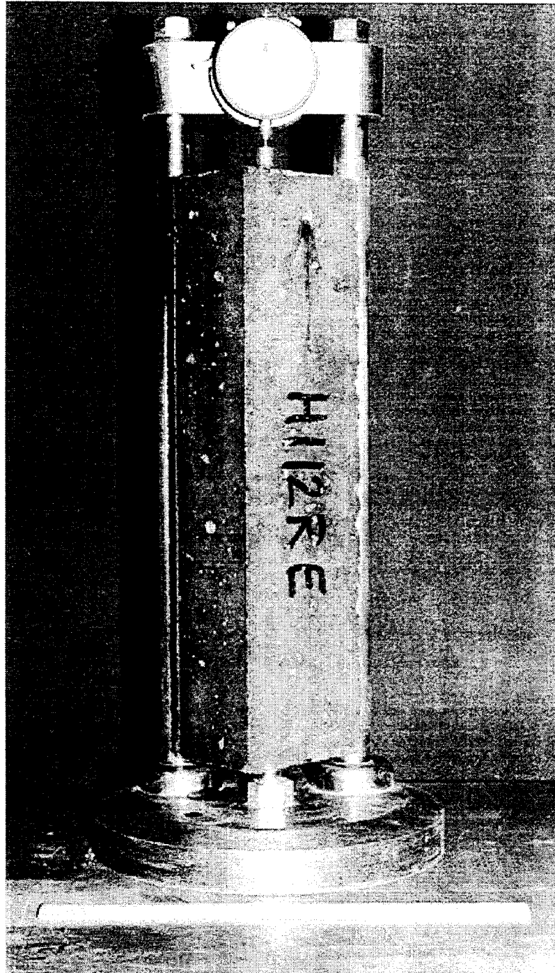
Figure 3.9 Length comparator: freeze-thaw test beam measurement
