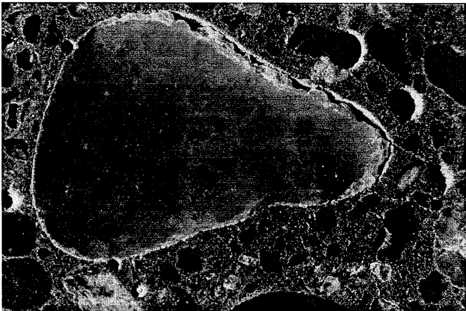
Figure 4.42 Phase II moist-cured round gravel with silica fume mix specimen
