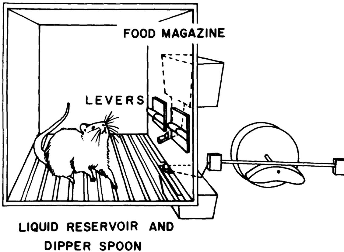
Figure 1. Schematic diagram of the operant conditioning chamber.
