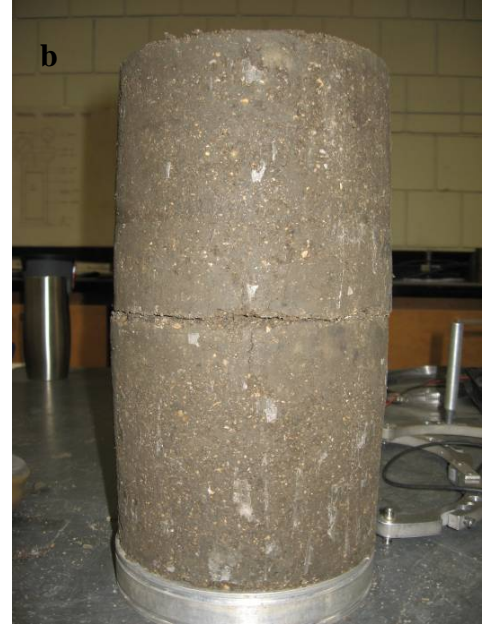
Figure A48. Pictures of 5% Foundry Sand + 95% Aggregate mixture failed specimen during resilient modulus and shear strength testing. Fig. A48a correspond to optimum moisture contents (<300 kPa suction), and Fig. A48b correspond to water content at 300 kPa suction.
