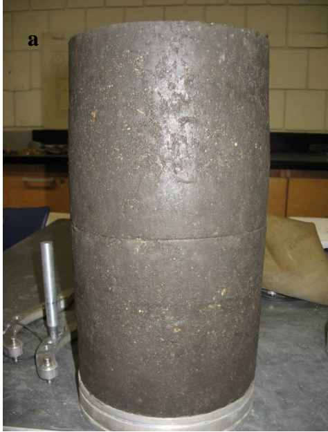
Figure A48. Pictures of 5% Foundry Sand + 95% Aggregate mixture failed specimen during resilient modulus and shear strength testing. Fig. A48a correspond to optimum moisture contents (<300 kPa suction), and Fig. A48b correspond to water content at 300 kPa suction.
