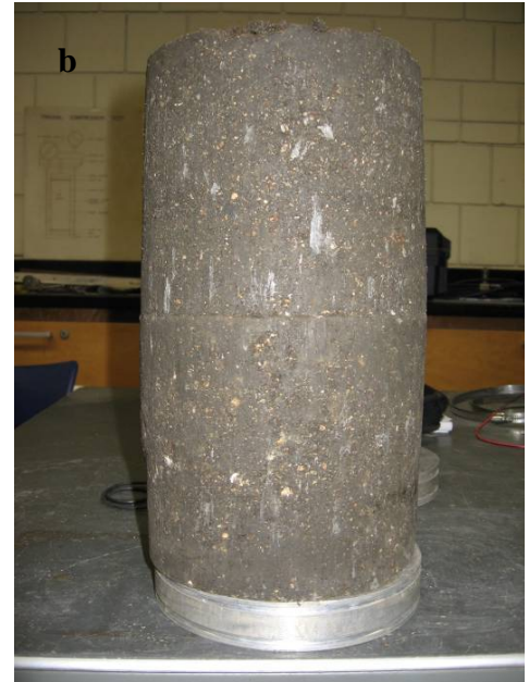
Figure A49. Pictures of 10% Foundry Sand + 90% Aggregate mixture failed specimen during resilient modulus and shear strength testing. Fig. A49a correspond to optimum moisture contents (<300 kPa suction), and Fig. A49b correspond to water content at 300 kPa suction.
