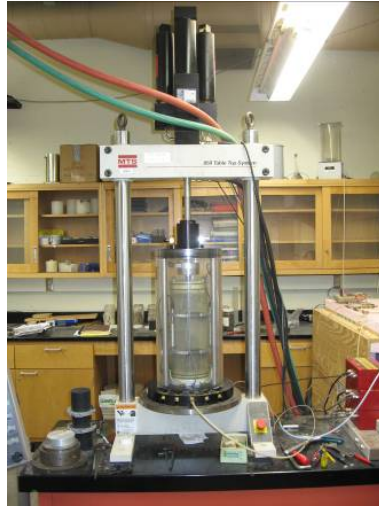
Figure 4.2 Loading frame and triaxial cell used for resilient modulus tests.
