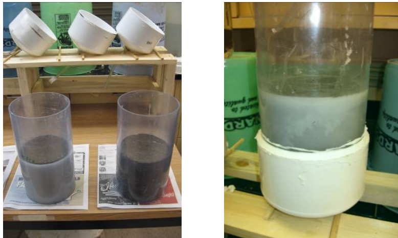
Figure 5.2 Assembly of specimens into leaching columns.
