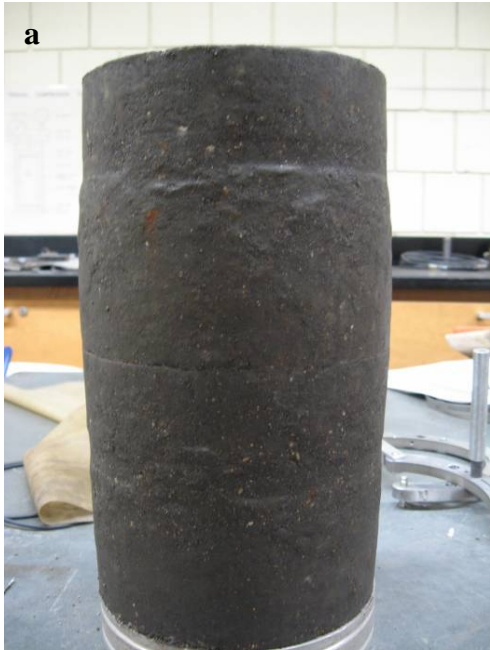
Figure A50. Pictures of 15% Foundry Sand + 85%Aggregate mixture failed specimen during resilient modulus and shear strength testing. Fig. A50a correspond to optimum moisture contents ( <300\text{ kPa} suction), and Fig. A50b correspond to water content at 300\text{ kPa} suction.
