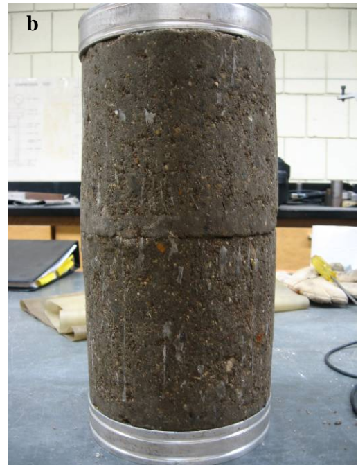
Figure A51. Pictures of 100%Aggregate failed specimen during resilient modulus and shear strength testing. Fig. A51a correspond to optimum moisture contents ( <300\text{ kPa} suction), and Fig. A51b correspond to water content at 300\text{ kPa} suction.
