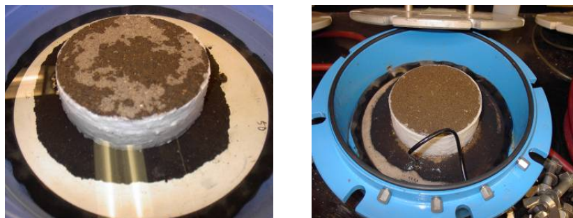
Figure 3.1 Paraffin coated specimen being saturated from bottom up under a small head of water and the placement of the specimen in the pressure chamber before the lid being bolted and air pressure being applied.
