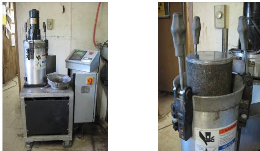
Figure 2.4 A gyratory compactor set-up.
