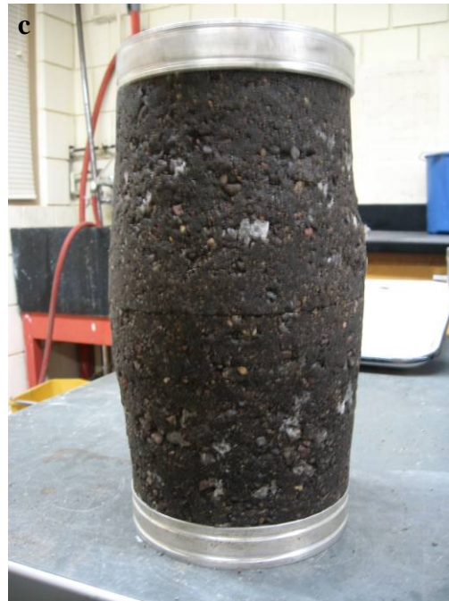
Figure A37. Pictures of 100% RAP mixture failed specimen during resilient modulus and shear strength testing for Fig. A37 a) and A36b) correspond to optimum moisture contents (<300 kPa suction), and Fig. A37c) correspond to water content at 300 kPa suction. Confining pressures were 1 psi for A37a and A37c specimens and 5psi for A37b specimen.
