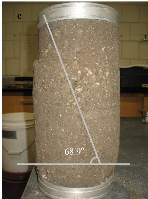
Figure A46. Pictures of 75% RCM + 25% Aggregate mixture failed specimen during resilient modulus and shear strength testing for Fig. A46 a) and A45b) correspond to optimum moisture contents (<300 kPa suction), and Fig. A46c) correspond to water content at 300 kPa suction. Confining pressures were 1 psi for A46a and A46c specimens and 5psi for A46b specimen.
