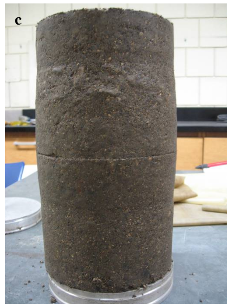
Figure A34. Pictures of 25% RAP +75% Aggregate mixture failed specimen during resilient modulus and shear strength testing for Fig. A34 a) and A34b) correspond to optimum moisture contents (<300 kPa suction), and Fig. A34c) correspond to water content at 300 kPa suction. Confining pressures were 1 psi for A34a and A34c specimens and 5psi for A 34b specimen.
