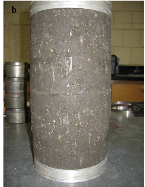
Figure A50. Pictures of 15% Foundry Sand + 85%Aggregate mixture failed specimen during resilient modulus and shear strength testing. Fig. A50a correspond to optimum moisture contents ( <300\text{ kPa} suction), and Fig. A50b correspond to water content at 300\text{ kPa} suction.
