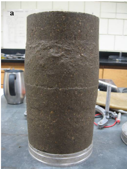
Figure A51. Pictures of 100%Aggregate failed specimen during resilient modulus and shear strength testing. Fig. A51a correspond to optimum moisture contents ( <300\text{ kPa} suction), and Fig. A51b correspond to water content at 300\text{ kPa} suction.
