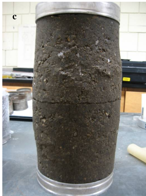
Figure A42. Pictures of 5% Fly Ash+ 75% RAP+20% Aggregate mixture failed specimen during resilient modulus and shear strength testing for Fig. A42 a) and A42b) correspond to optimum moisture contents (<300 kPa suction), and Fig. A42c) correspond to water content at 300 kPa suction. Confining pressures were 1 psi for A42a and A42c specimens and 5psi for A42b specimen.
