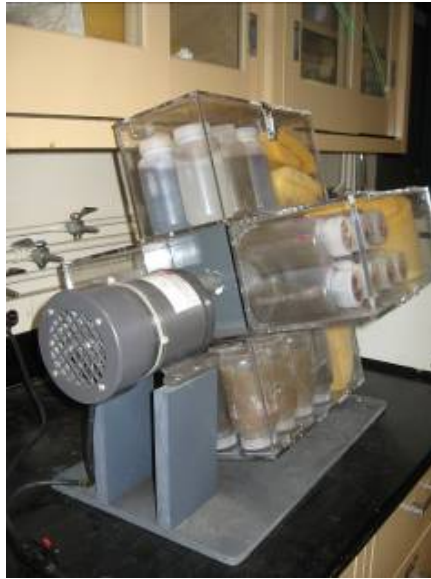
Figure 5.1 A rotary end-over-end mixer used for mixing recycled-aggregate mixtures with Milli-Q water in a batch test.
