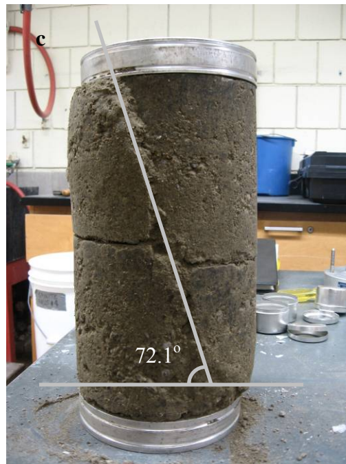
Figure A41. Pictures of 15% Fly Ash+50% RAP+35% Aggregate mixture failed specimen during resilient modulus and shear strength testing for Fig. A41 a) and A41b) correspond to optimum moisture contents (<300 kPa suction), and Fig. A41c) correspond to water content at 300 kPa suction. Confining pressures were 1 psi for A41a and A41c specimens and 5psi for A41b specimen.
