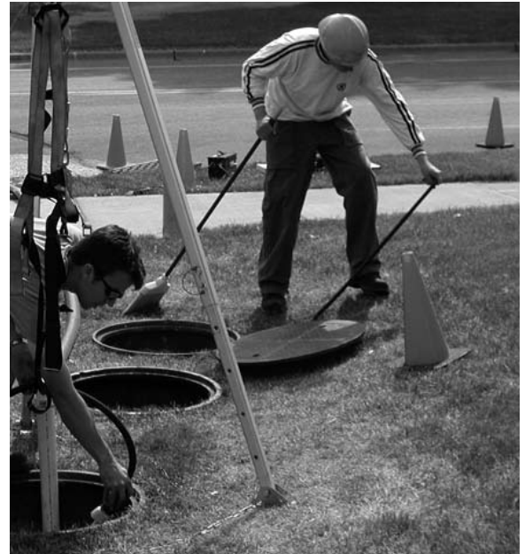
Researchers tested storm water treatment devices to gauge how well they remove sediment.
