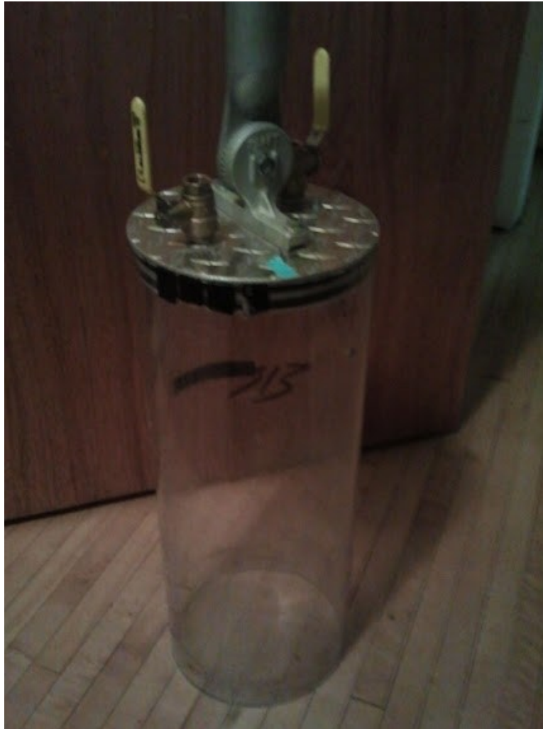
Figure 4. Sediment core tube attached to sediment corer and drive rod.
