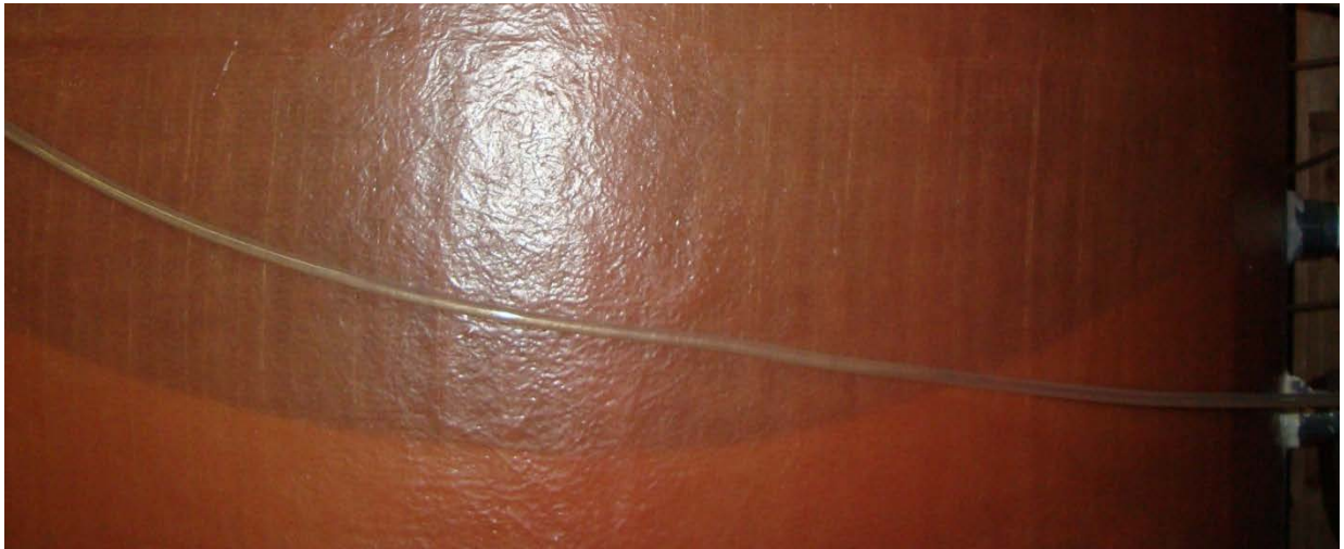
Figure 3-11: The once level sediment bed, shown drastically altered after Test 1. View from outside of the sump.
