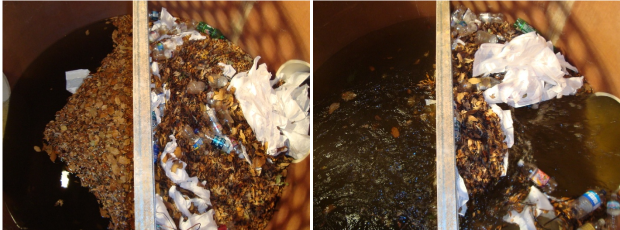
Figure 3-12: (Left) loading phase of Test 2. (Right) washout phase of Test 2. The water flow is from right to left.
