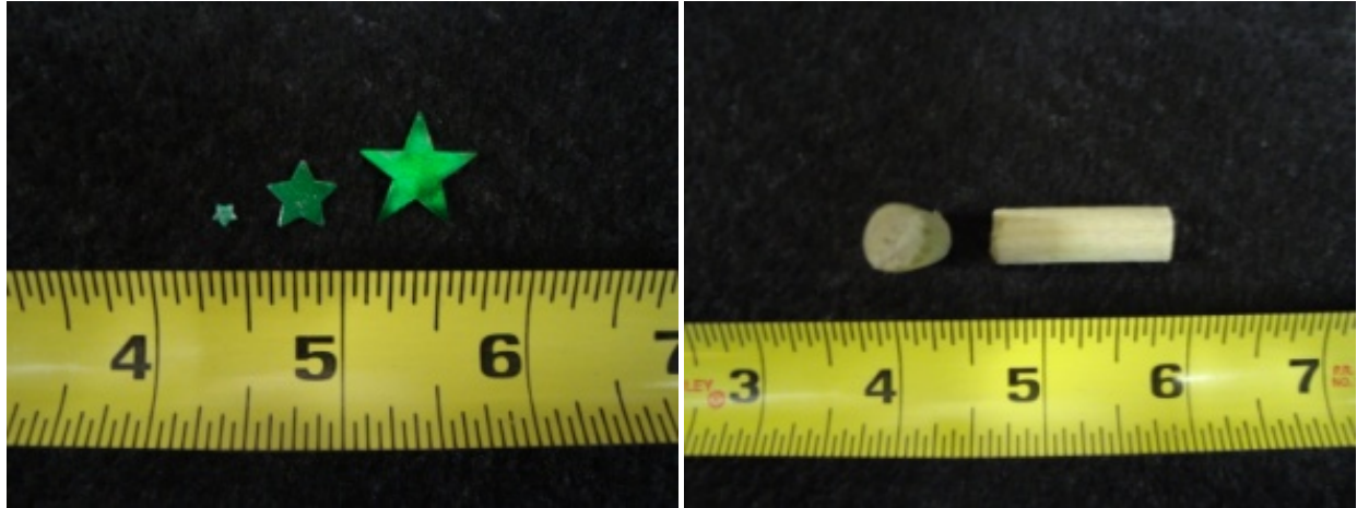
Figure 3-3: Simulated debris mixture (left) 80% confetti (right) 20% wood dowels.
