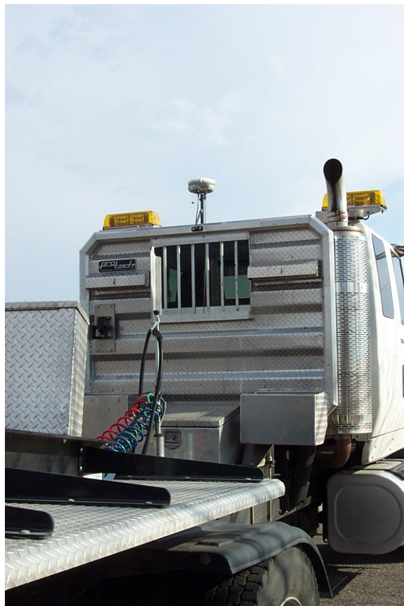
Figure 2.17: Differential GPS system located above tractor cab.
