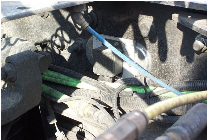
Figure 2.5: Accelerometer at front left top of tractor.
