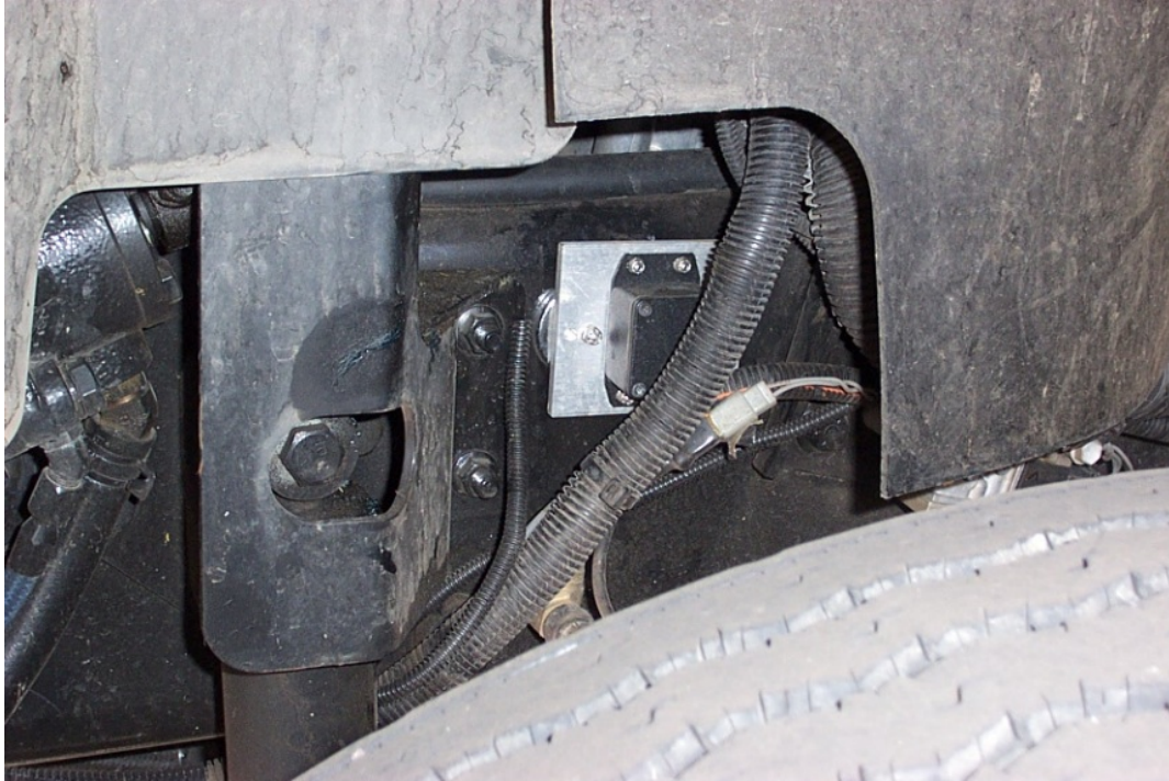
Figure 2.8: Accelerometer on tractor body near the front (steering) axle.
