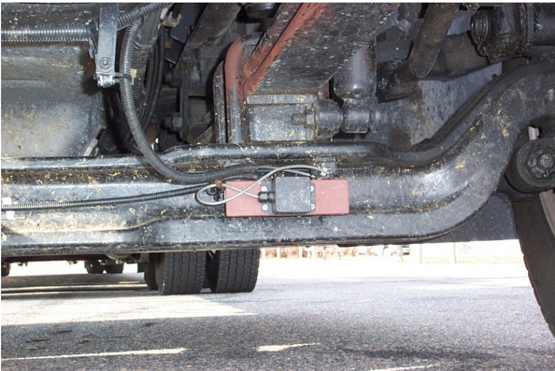
Figure 2.7: Accelerometer on front (steering) axle of tractor at bottom left.
