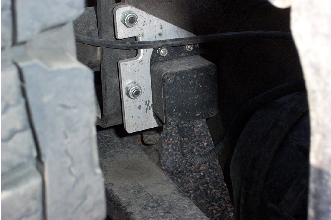
Figure 2.6: Accelerometer at second axle of tractor on bottom right.
