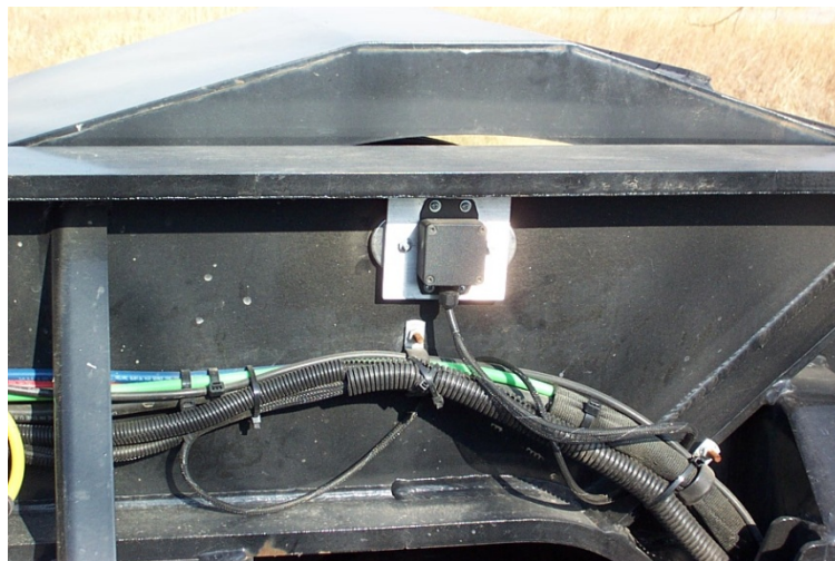
Figure 2.1: Accelerometer at top left near the front of trailer (TLF2 location).
