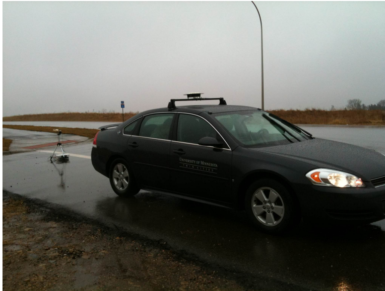
Figure 6.6: Instrumented testing vehicle at northeast starting point of "S" route. The base receiver antenna is on the tripod behind the vehicle.
