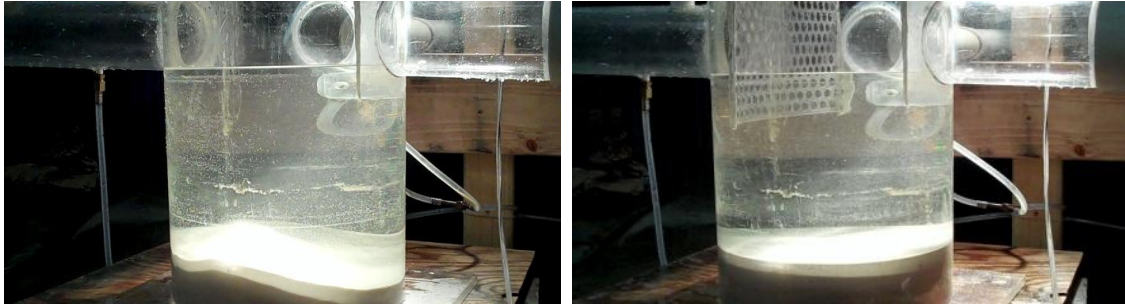
Figure 3-3: Post washout test on the 1×1-90 Degree Outlet sump without a SAFL Baffle and with a SAFL Baffle oriented at 90 degrees to the inlet pipe
