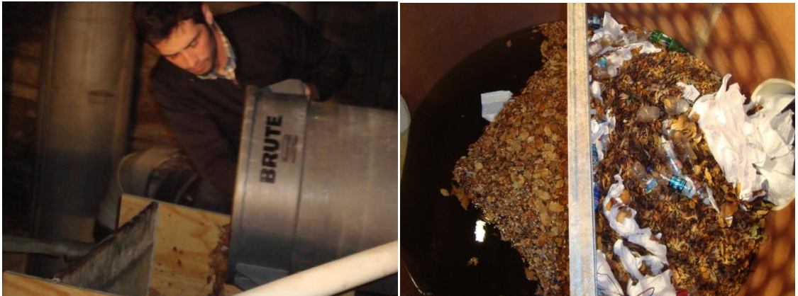
Figure 2-4: (Left) Loading simulated debris upstream of the manhole sump. (Right) Water leaving the sump's outlet and traveling through the tail box, where debris is collected.
