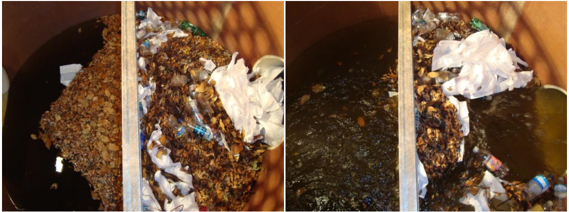
Figure 2-7: (Left) Loading phase of Test 2. (Right) Washout phase of Test 2. The water flow is from right to left.
