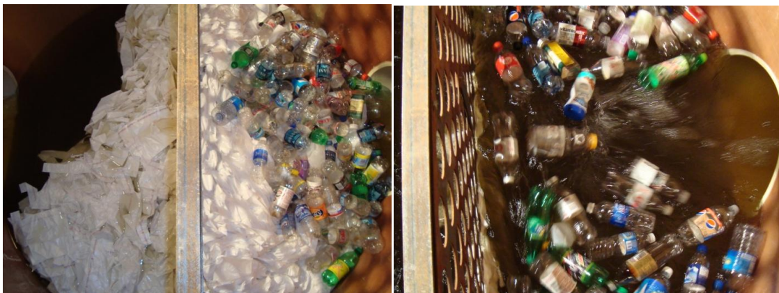
Figure 2-10: (Left) Loading phase of Test 1. (Right) Washout phase of Test 1. The flow is from right to left.
