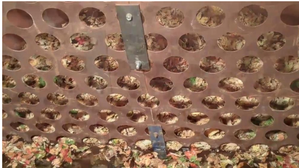
Figure 2-9: Test 2 from the 6×3 washout testing series during its loading phase. The view is from near the outlet pipe, looking upstream.
