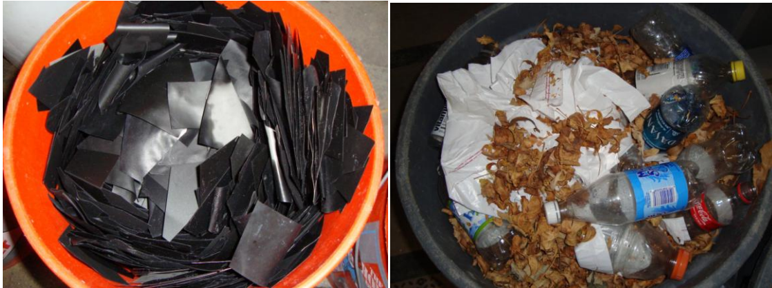
Figure 2-5: Vinyl leaves, plastic grocery bags, and plastic bottles used as simulated debris
