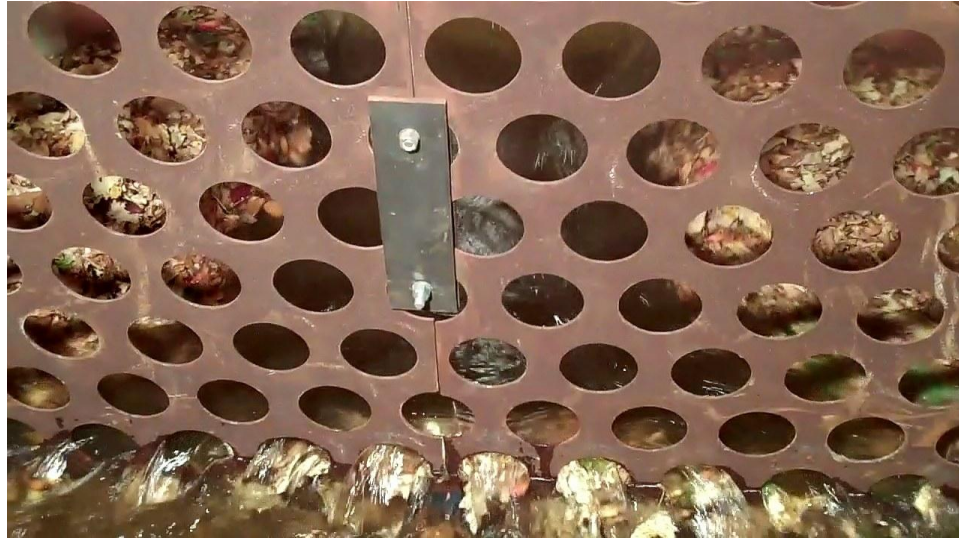
Figure 2-10: Test 2 from the 6×3 washout testing series during its washout phase. The view is from near the outlet pipe, looking upstream.
