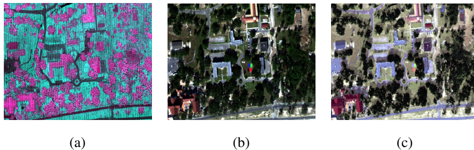
Figure 6.1: Fusion of HSI and LiDAR data from the Gulfport scene. (a) Depth-intensity-average map from LiDAR. (b) False color RGB from hyperspectral scene. (c) False color RGB from HSI-LiDAR fused scene. (This is a color figure.)
