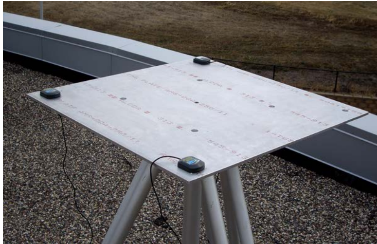
Figure 3.6: Phase center calibration test setup
