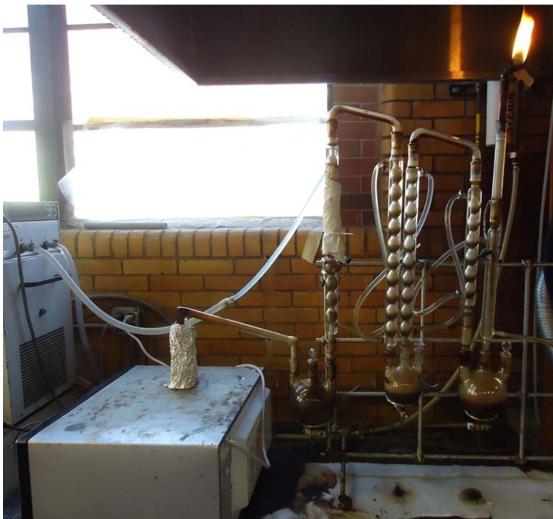
Figure 3.5 The microwave-assisted pyrolysis system
