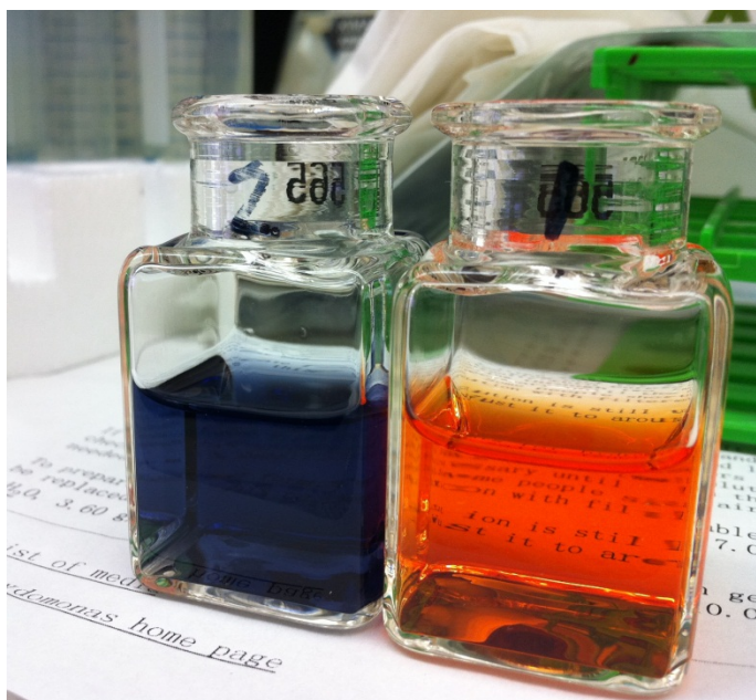
Figure 3.4 The sample (left) and the blank (right) of zinc ion concentration measurement
