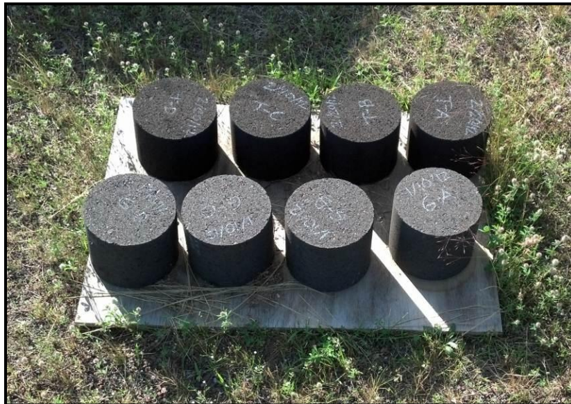
Figure 18: Specimens placed at closed weigh station on Interstate 35 for field conditioning
