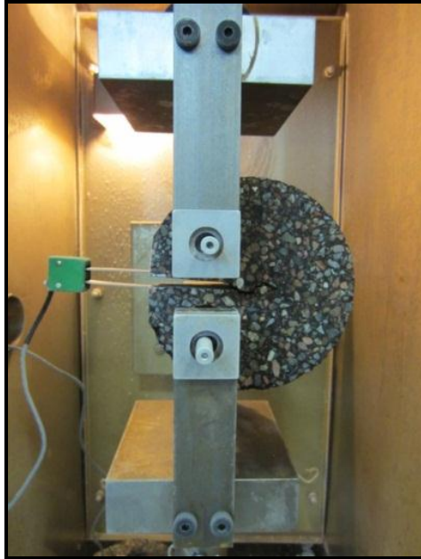
Figure 15: DCT specimen placed into loading frame
