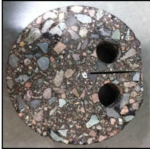
Figure 14: DCT test specimen
