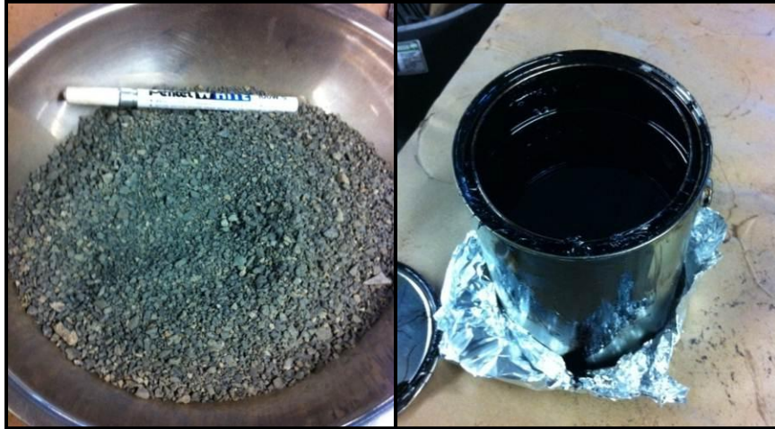
Figure 9: Minntac Coarse Tailings and binder prepared for mixing
