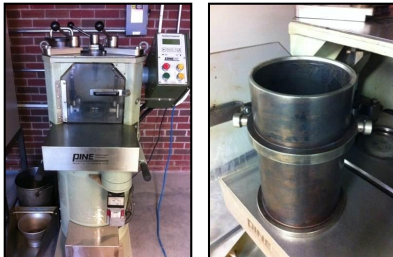
Figure 11: Pine Superpave gyrator compactor and steel mold
