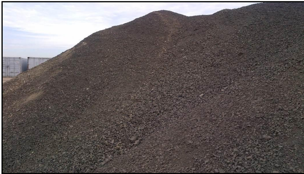
Figure 2: Taconite tailings used for railroad ballast outside of Minot, ND (Enbridge)
