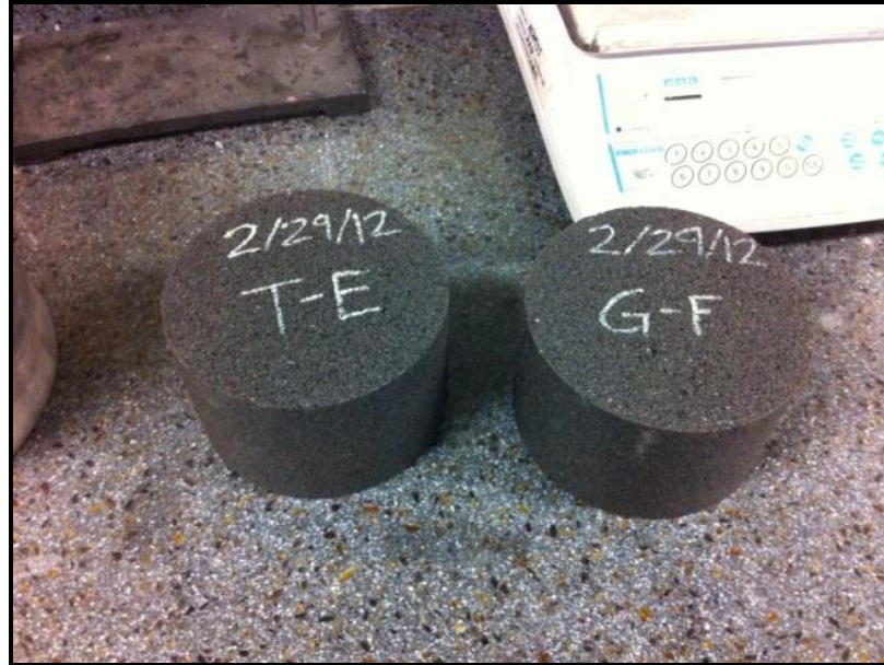
Figure 12: Compacted asphalt specimens
