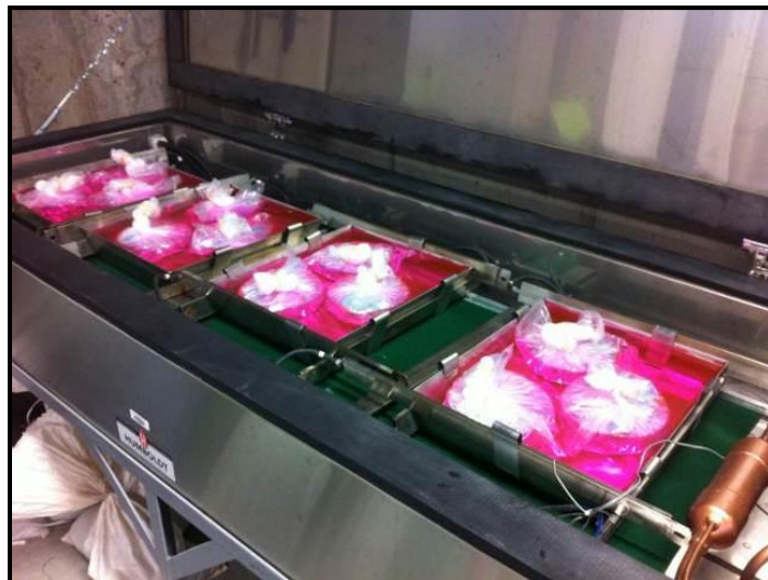
Figure 17: DCT samples prepared for multiple freeze-thaw conditioning
