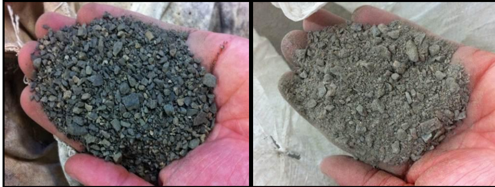
Figure 6: Visual comparison of taconite tailings (left) and granite aggregate (right)
