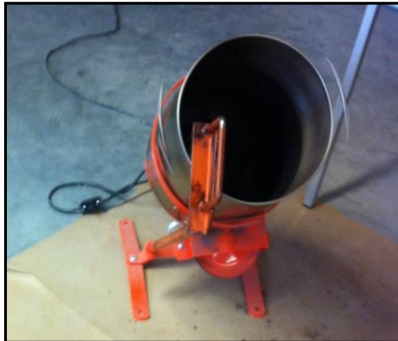
Figure 10: Mixing of aggregate and binder
