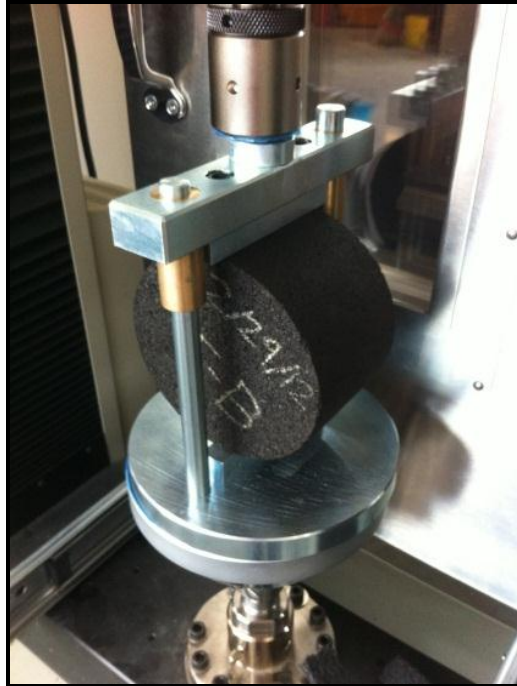
Figure 13: AASHTO T-283 test setup
