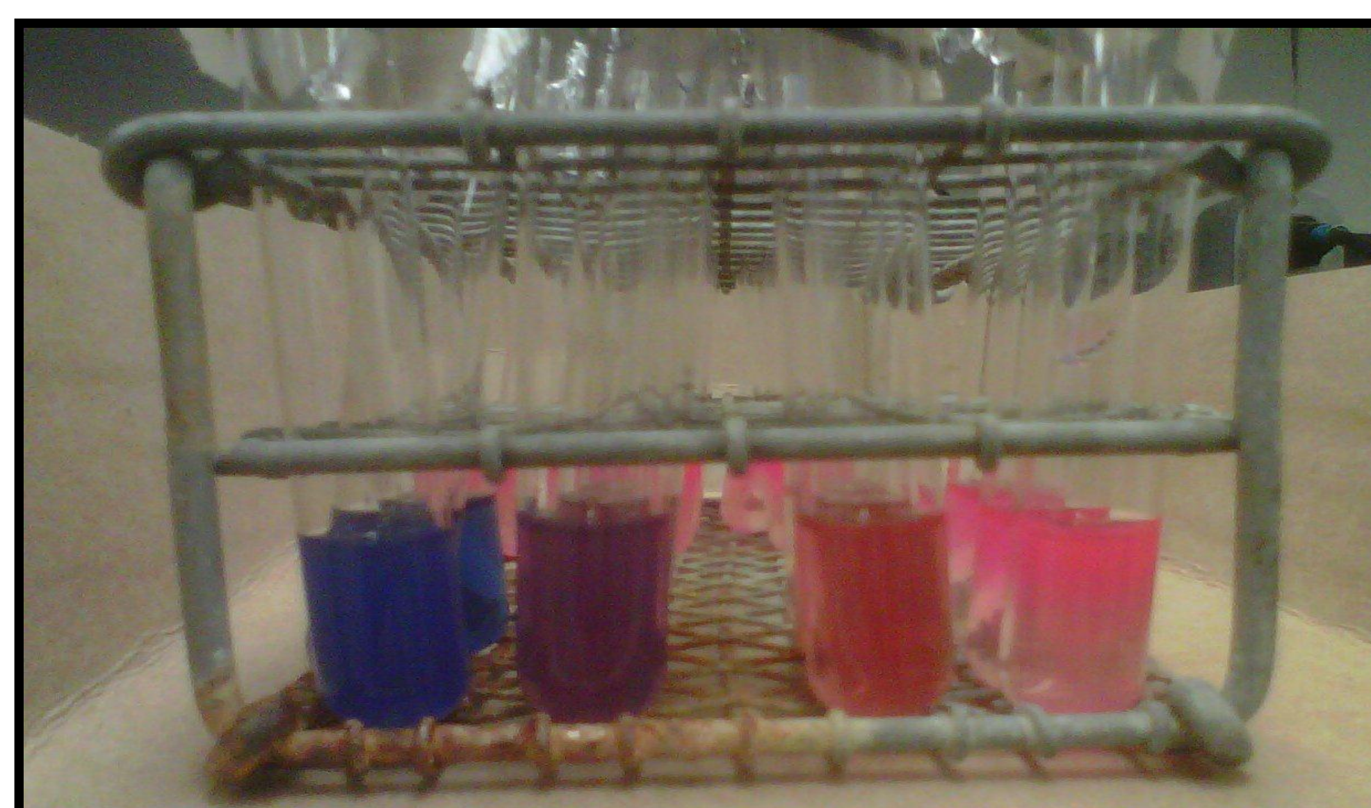
Fig.1. Sample cuvettes containing differing concentrations of PCNB in solution with V8 broth, P.sojae zoospores, and Alamar Blue. (From left to right) Cuvettes contain 500, 250, 125, and 0 ug/ml of PCNB.
