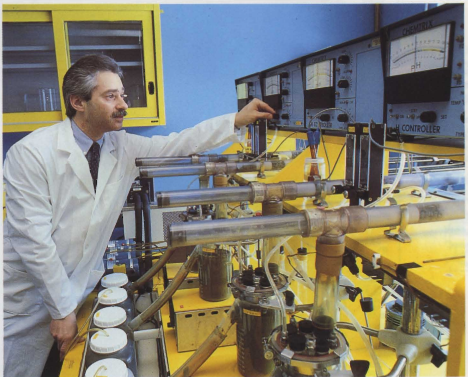
Marshall Stern's laboratory simulates the digestive process of cows with banks of glass "digestors" processing different feeds. Monitors record the process of protein breakdown within the artificial stomachs.
