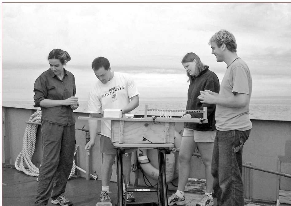
Researchers (from left to right) Ann M. McNally, Douglas E. Latch, Kristine H. Wammer, and Jeffrey J. Werner measure photochemical kinetics in samples arranged in a row of quartz test tubes on the deck of the Blue Heron.
