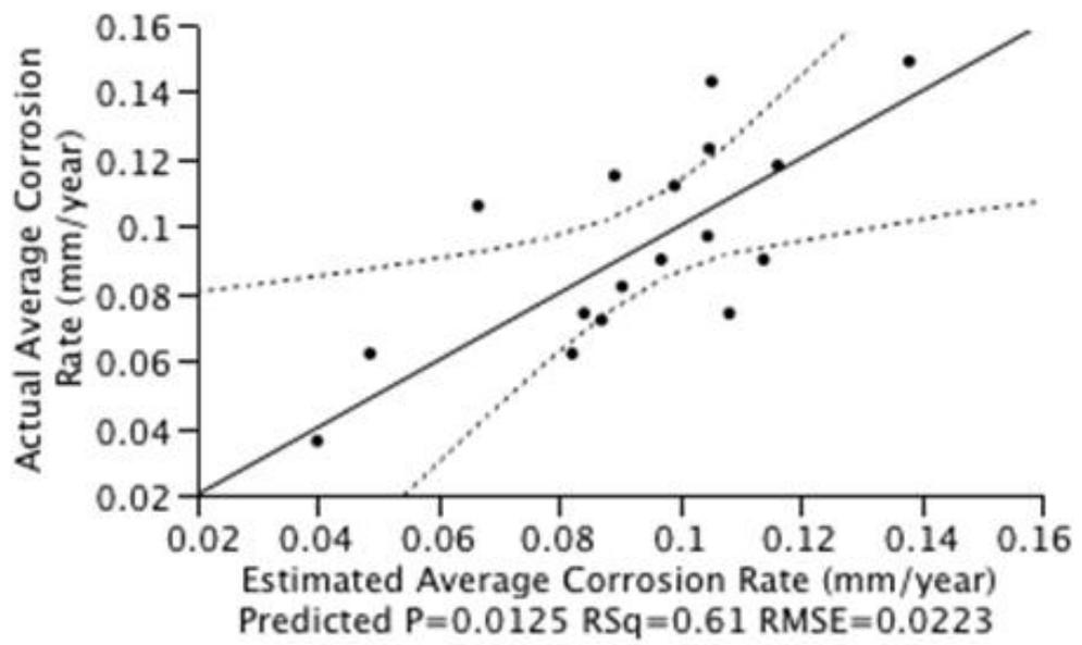
Table 6. Comparison of long-term corrosion rates to corrosion rates predicted by the multiple regression model. The standard deviation (SD) of actual corrosion rate measurements and 95% confidence interval (CI) of predicted corrosion rates estimated by the model are shown. ND indicates that a long-term corrosion rate could not be determined at the Two Harbors site because the age of the steel structure was unknown.
