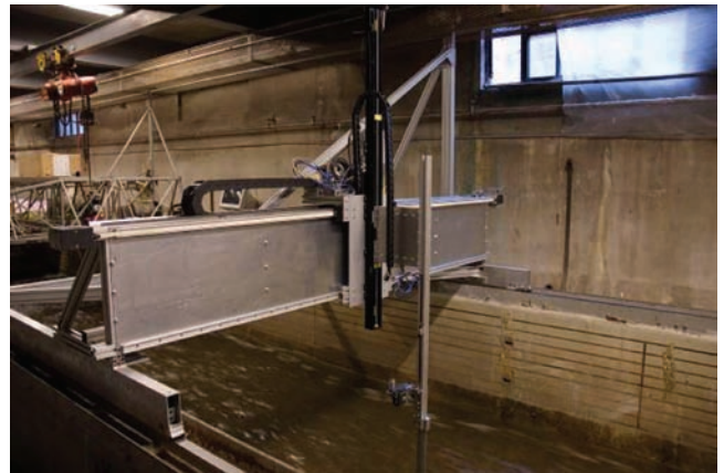
Figure 2. Three-axis automated data collection carriage.
