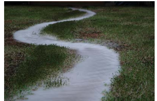
Figure 2. Image of a self-formed, laboratory scale meandering stream. The channel is approximately 15 cm wide.
