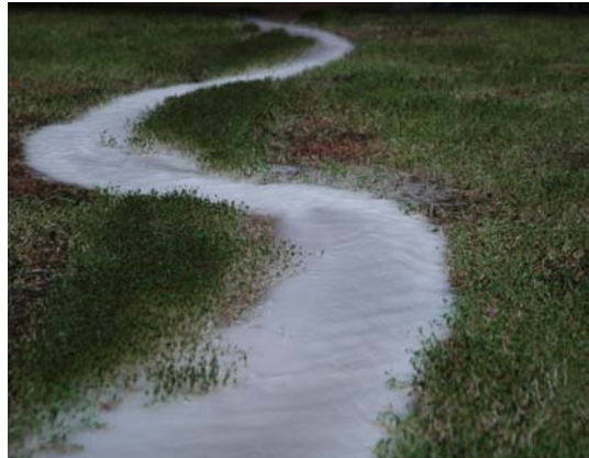
A self-formed, meandering channel created in a flume using alfalfa sprouts to provide strength to banks and bars.
