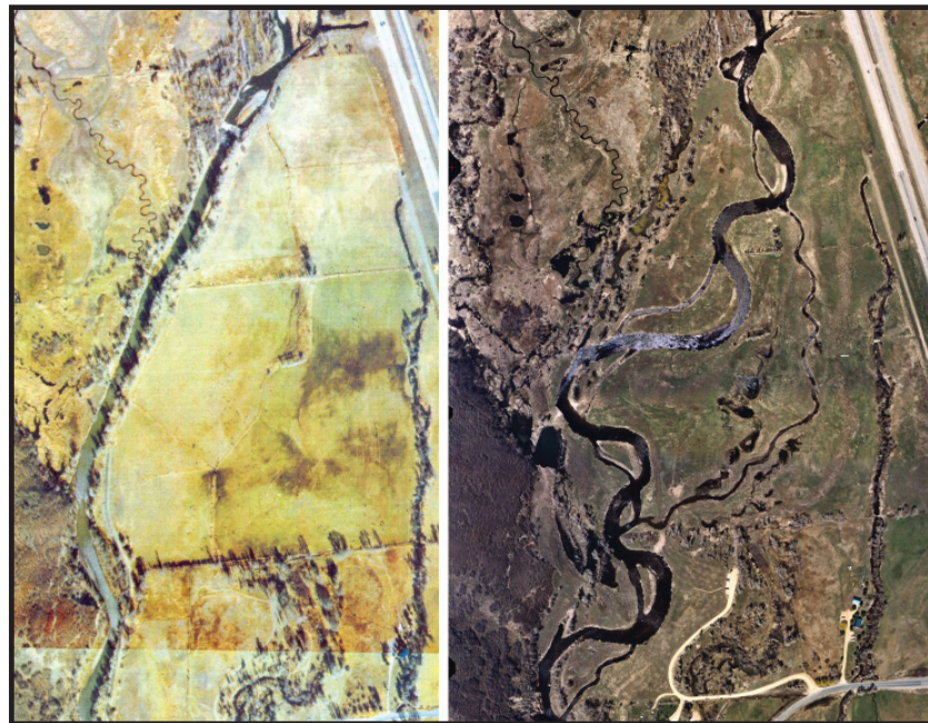
Aerial photographs of Reach 7 of the Middle Provo. Left: photo taken before construction (1999) and shows how channelized the river had become. Right: Photo taken after reconstruction (2004) of meanders and side channels, and shows the wide corridor now available to the river. Photos courtesy of PRRP.
