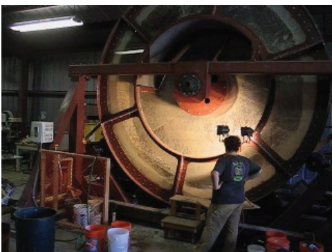
Figure 7: The 4 m diameter vertically rotating drum at the Richmond Field Station.
