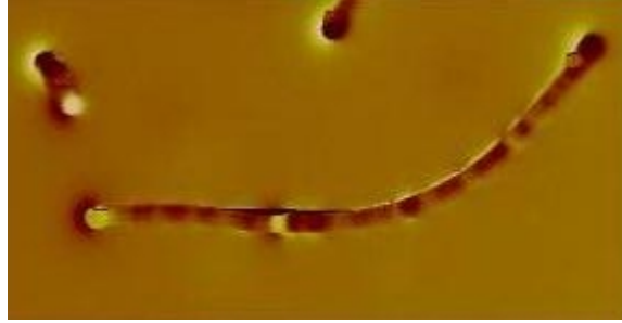
Figure II.3: Bent wires of Galfenol
