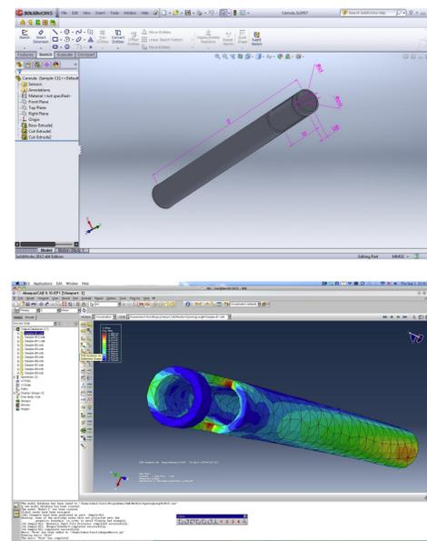
The SolidWorks model was automatically updated during the design. The Abaqus output shows the simulation results of a stainless steel cannula with a fixed proximal end and a concentrated load applied close to the tip.
