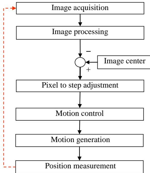
Figure 14, Motion control and tracking realization diagram
