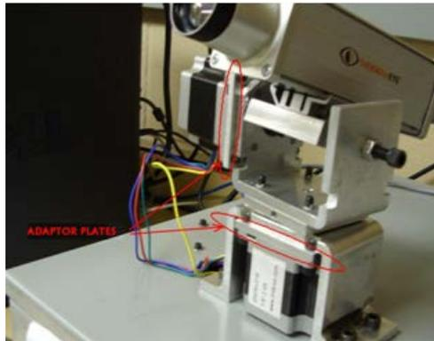
Figure 6 - Camera installation
