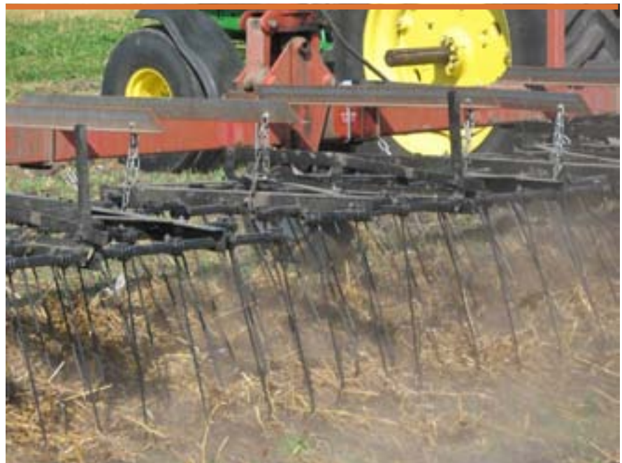
Figure 6-10. Large amounts of residue can interfere with flex tine weeders.
