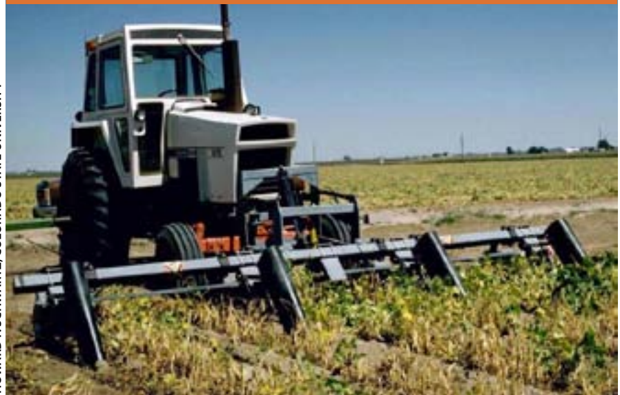
Figure 14-2. Tractor-driven cutter used to harvest dry beans.
