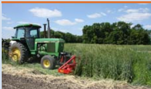
Figure 13-12. A roller-crimper rolling down a biculture of winter rye and hairy vetch while planting soybeans.
