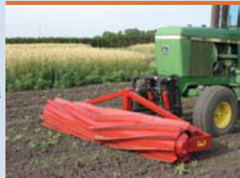
Figure 13-11. Roller-crimper attached to the front of a tractor.
