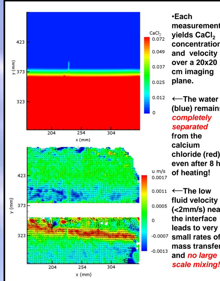
•Each measurement yields  $\text{CaCl}_2$  concentration and velocity over a 20x20 cm imaging plane.
