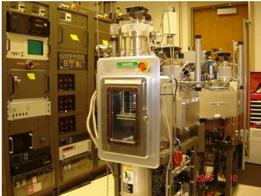
Fig.2.1 Shamrock Sputtering System, with load/unload chamber; transfer chamber and main deposition chamber with six targets.
