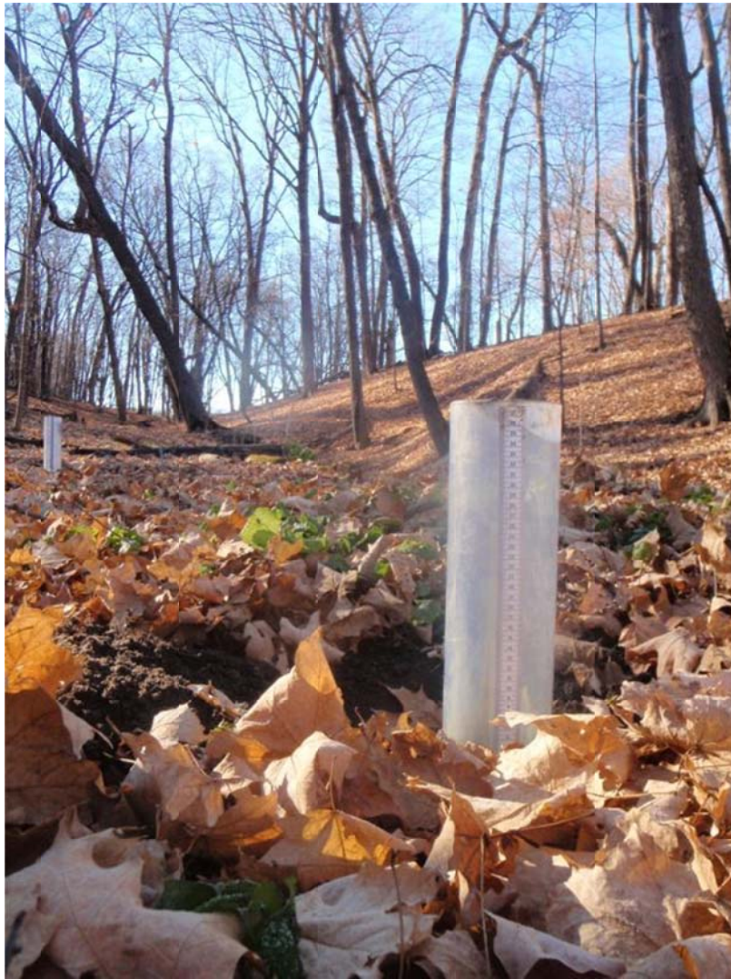
Figure 3.1 The Modified Philip-Dunne (MPD) Infiltrometer in place for K measurement.
