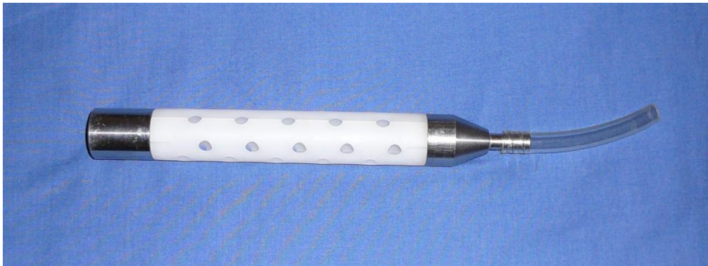
Figure 5. Manufacturer-recommended sampling manifold, with a diameter of approximately 2.5 cm (1 in)
