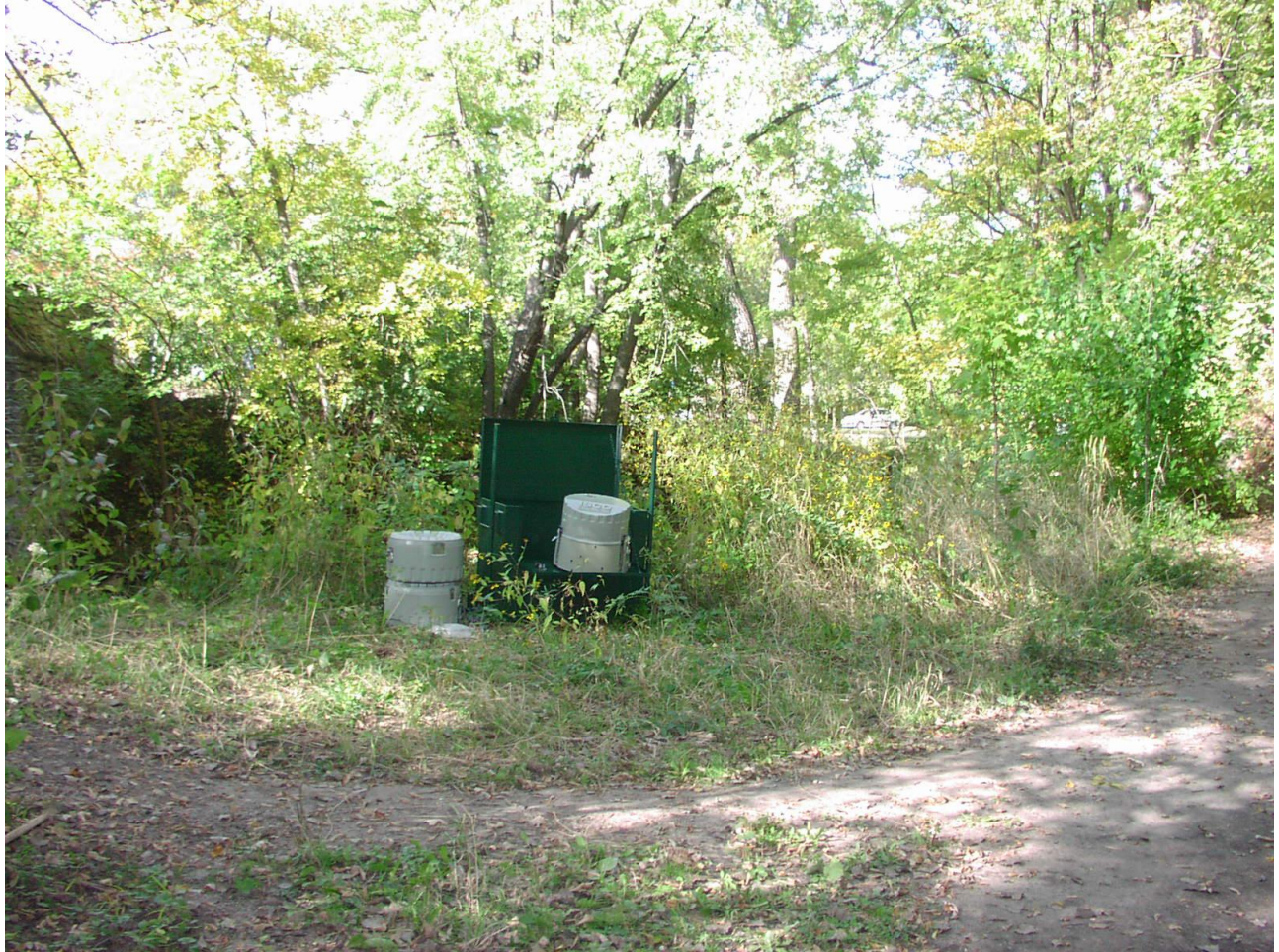
Figure 15. Equipment set up at Commonwealth Site in St. Paul, MN with two automatic samplers and a protective metal box.
