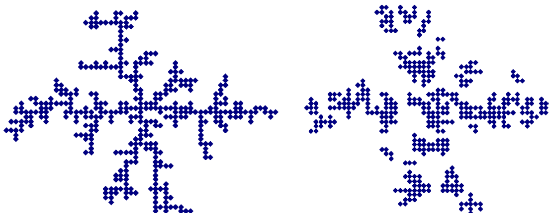
Figure 7.4 Aggregate composed of 400 square particles with equivalent faces before (left) and after (right) 200 coalescence cycles with an unstick chance of 5%.
