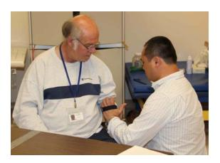
Figure 3. Shoulder flexion hand-held dynamometer strength testing.
