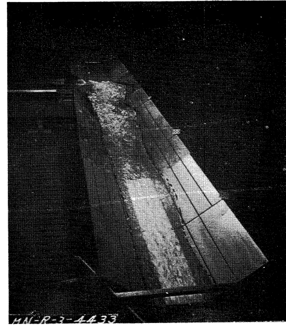
(b) This represents conditions corresponding to prototype flows of 207 cfs in the inlet main and 181 cfs in the lateral.
