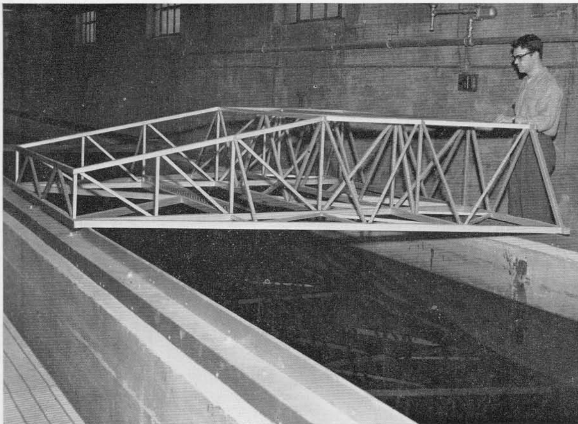
Fig. 9—Towing Carriage Frame Prior to Installation of Wheels and Drive System. Over-all dimensions are length—12 ft, width—10 ft, and height—30 inches. Unit is constructed of square tubing varying in size from \frac{7}{8} inch to 1\frac{1}{4} inches.
