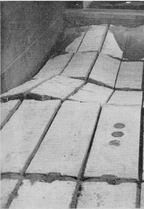
Fig. 5—Tests of Concrete Mattress for River-Bank Protection. Upper photograph prior to test. Lower photographs show settlement of mattress as a result of scouring of sand bed beneath mattress by the flowing water, and observer looking through glass sidewall during test with hydrodynamic pulsimeter in stream above mattress.
