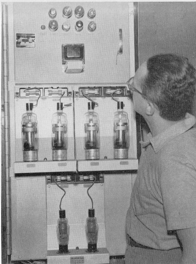
Fig. 11—Thy-mo-trol Power Supply and Control System. Left: View of Thyatron tubes. Right: Interior of cabinet, showing control elements.
