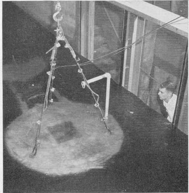
Fig. 5—Tests of Concrete Mattress for River-Bank Protection. Upper photograph prior to test. Lower photographs show settlement of mattress as a result of scouring of sand bed beneath mattress by the flowing water, and observer looking through glass sidewall during test with hydrodynamic pulsimeter in stream above mattress.
