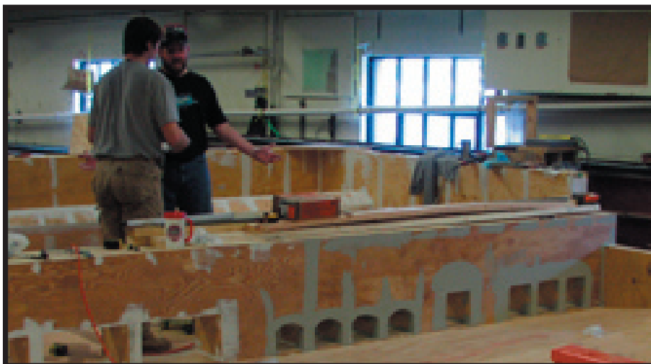
Dick Christopher and Nate Flemming discuss construction of the fish bypass system model. They're standing just behind the gatehouses.
