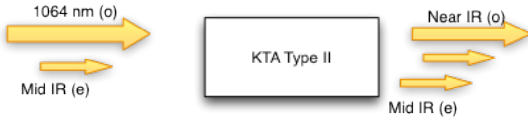
Figure 6.9. Optical Parametric Amplification of Mid IR in a KTA Crystal.
