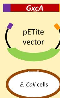
**3. Transform** by heat shock. The gene is inserted into the vector by homologous recombination within the cells. Select for recombinants on kanamycin agar plates.
