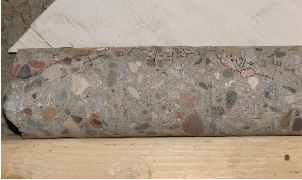
Figure E3: Crack widths marked on core specimen in pencil
