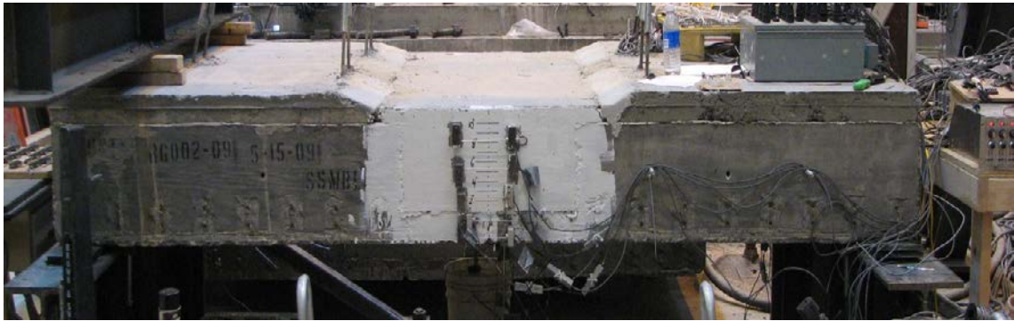
Figure 6.1.5: Elevation view of SSMBLG3-HighBars and increased deck depth to provide additional cover for the shrinkage reinforcement in the deck
