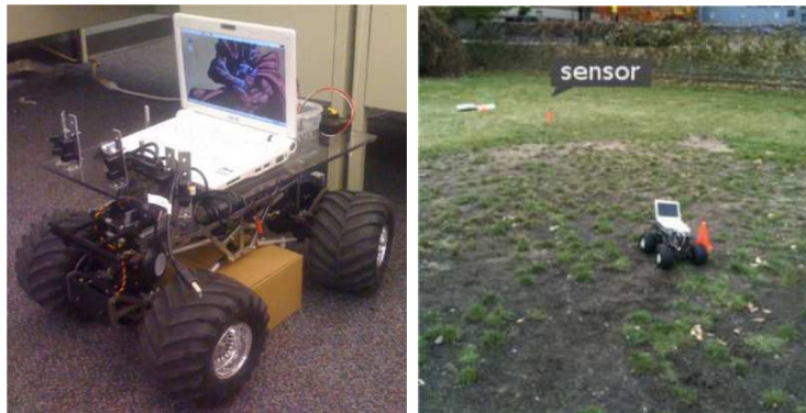
Figure 3.13: Left: Cyclops robotic platform developed for data muling. Right: A data mule system together with sensors.
