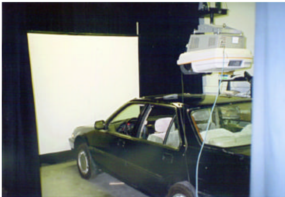
Figure 2.1. Human Factors Research Laboratory's Front-Projection Driving Simulator
