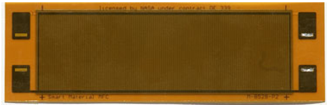
Figure 2.4 Photograph of Smart Material™ MFC-PZT with d_{31} effect [10].
