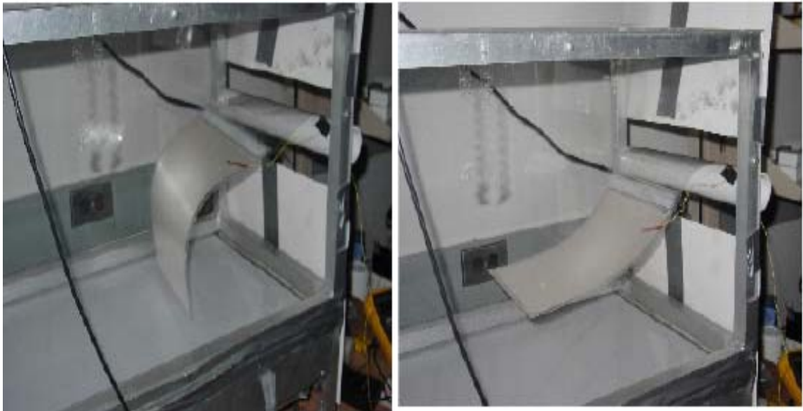
Figure 3.1. Photograph of PVDF down stroke (left) and upstroke (right) [5].
