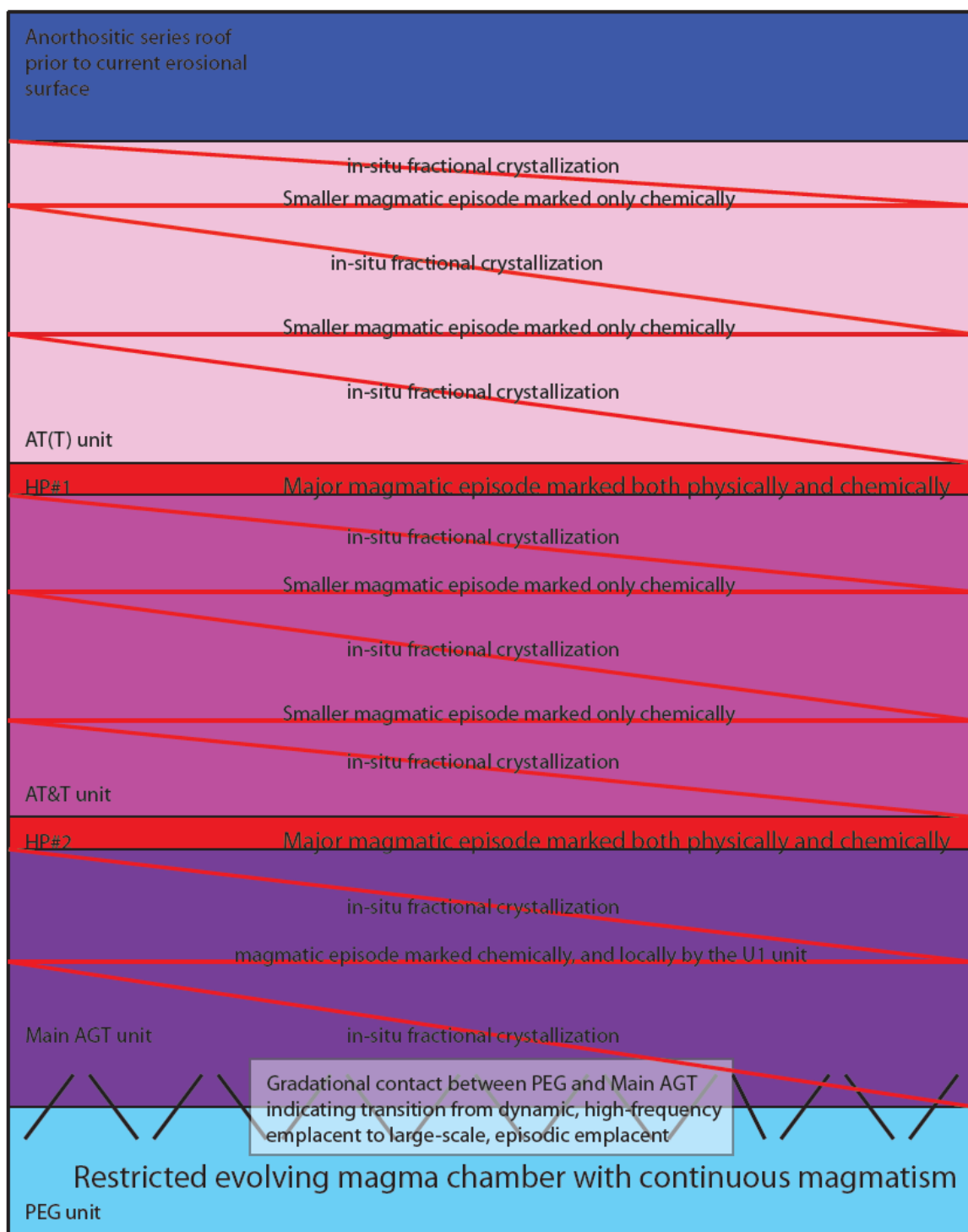
Figure 64: Model for emplacement of the upper zone, featuring in situ fractional crystallization with episodic magma recharge.
