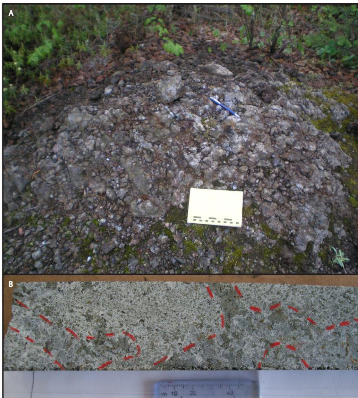
Figure 35: A. the BH unit in outcrop with a weathered, gossan-stained, grussy appearance, (Outcrop station 60407-01; Appendix I); and B. the BH unit in drill core displaying heterogeneity in lithology and grain size with sharp internal contacts; red dashed lines outline lithologies; Drill hole MEX-61 – depth 3384 feet.
