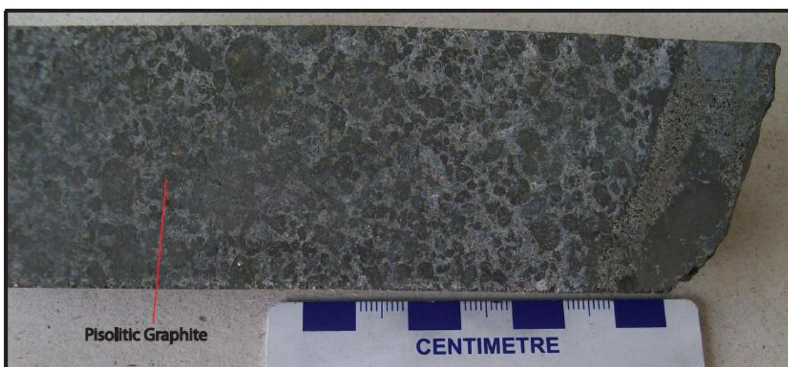
Figure 25: Metasedimentary inclusion featuring globular graphite with a matrix of quartz; Drill core MEX-47 - depth 1809 feet.
