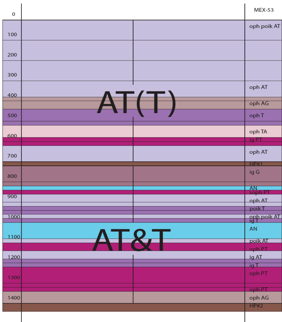
Figure 63: Profile through the AT&T and AT(T) units taken from drill hole MEX-53, illustrating randomly alternating lithologies and textures (T – troctolite, AT – anorthositic troctolite, PT – augite troctolite, TA- troctolitic anorthosite, G – gabbro, AG – anorthositic gabbro, AN – anorthosite, ig – intergranular, oph – ophitic, poik – poikilitic olivine).
