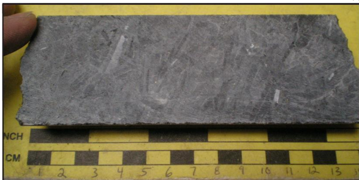
Figure 30: Well foliated anorthosite of the AN-G unit; Drill hole MEX-51 – depth 2401 feet.
