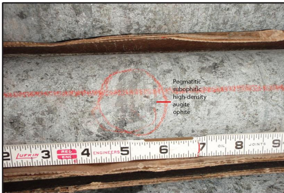
Figure 41: The PEG unit in drill core composed of coarse-grained augite troctolite with pegmatitic, subophitic oikocrysts of augite; Drill core MEX-133M – depth 789 feet.
