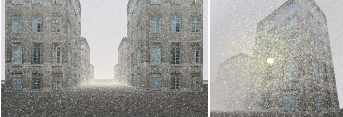
Figure 3.7: Color screen captures from the current snow rendering system. One million particles were released into each scene. The right image shows direct use of the phase function in which a streetlight illuminates particles as they pass by the viewer.
