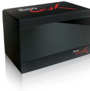
Picture 5: Picture of Ibeo Lux. The sensor is small, H85 x W128 X D83mm
