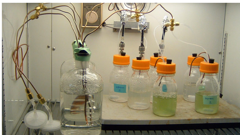
Figure B-1. Experimental apparatus used for supplying LB400 with a constant stream of reduced-oxygen gas. In this photo, two of the reactors (and one control) were used to measure the growth of Synechocystis sp. PCC 6803 (a blue-green algae) and three were used to measure LB400 growth on biphenyl, which necessitated a carbon trap at the reactor exit.
