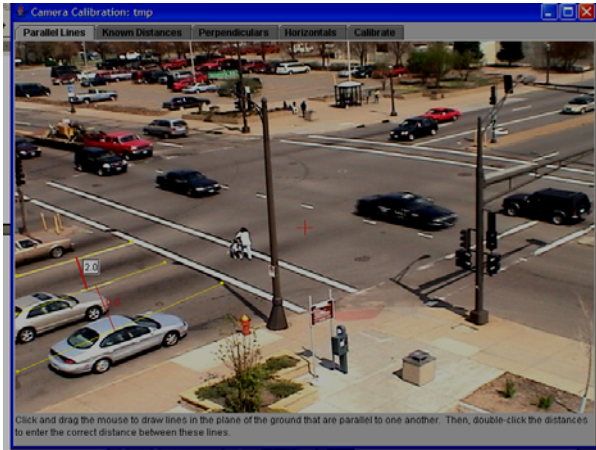
Fig. 3.7(a) Setting the parallel lines. The parallel lines are indicated along with the distance between them by the connecting lines. The distance between parallel lines or lanes can be altered by the user.
