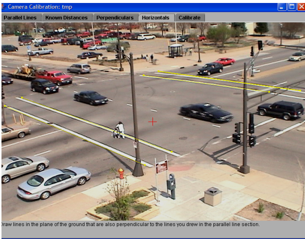
Fig. 3.7(c) Horizontal; the horizontal lines are indicated.
