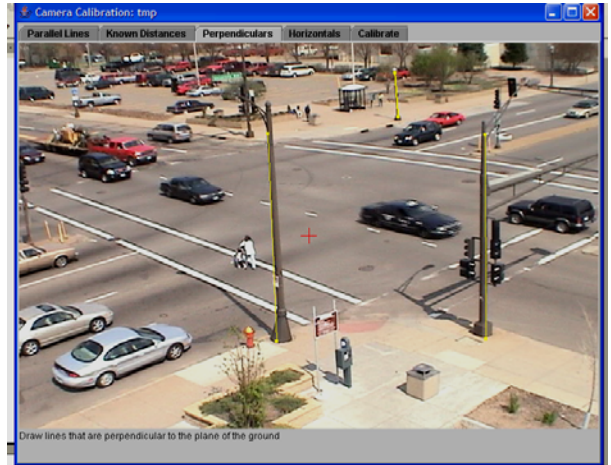
Fig. 3.7(b) Perpendiculars; the perpendiculars are indicated by the lines on the poles.
