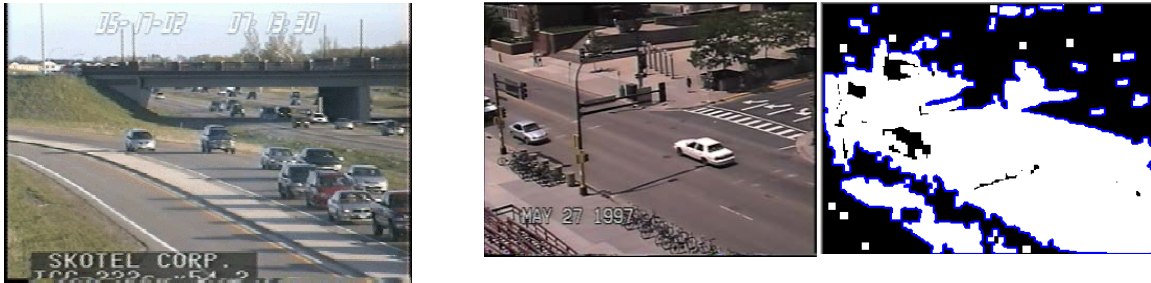
(a) Poor placement such as oblique views can result in large occlusions between targets. Large background occlusions, spatial resolution, and illumination changes
