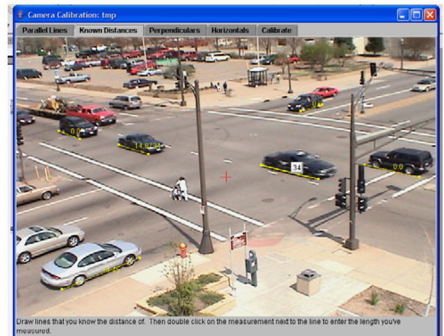
Fig. 3.7(d) Known measurements; known measurements with their corresponding true distances (in ft) are indicated as shown
