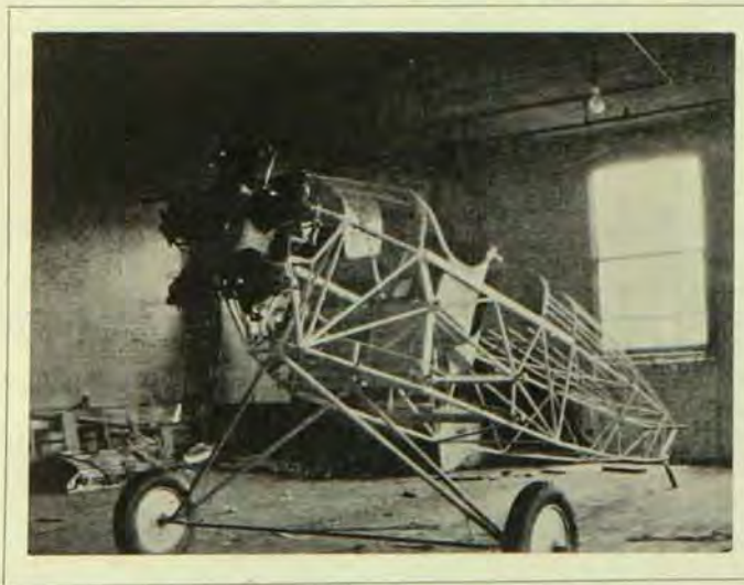
"The fuselage of the Mohawk plane is of the electrically welded tube type. This in turn is covered with heavy cloth, the whole of which is painted with aluminum paint.
